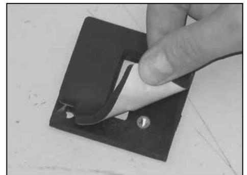
17. Install the provided gasket onto the mass air sensor adapter.
