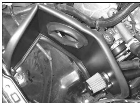
14. Install the heat shield into the vehicle and secure with the provided hardware.
