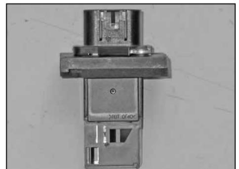
19. Install the mass air sensor into the K&N® mass air sensor adapter. Secure with the provided hardware.
