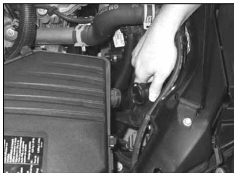
3. Depress the locking ring on the air pump fresh air inlet tube. Disconnect the fresh air inlet tube from the upper air box.
