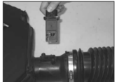
18. Remove the mass air sensor from the vehicle as shown.
