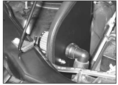
15. Secure the air pump fresh air tube to the adapter as shown.
