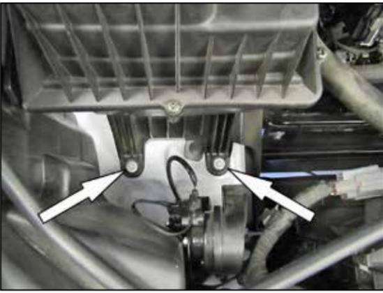
7. Remove the two bolts securing the air filter housing to the inner fender.
