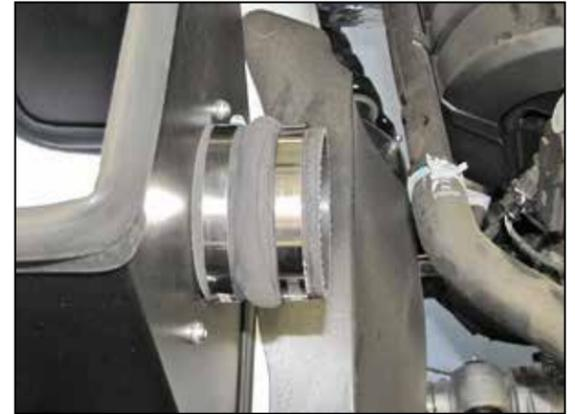
19. Install the provided coupling hose (08699) onto the filter adapter and secure with the provided hose clamp.
