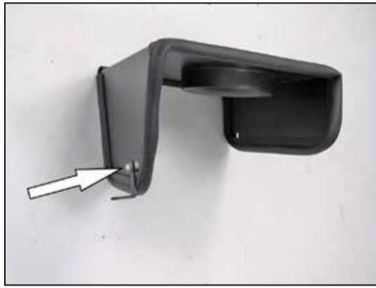
12. Install the heat shield mounting bracket (070712A) onto the heat shield using the provided hardware and spacer.
