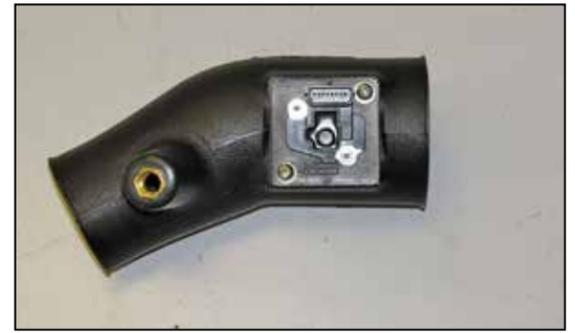
17. Install the mass air sensor into the K&N adapter and then install the assembly into the K&N intake tube and secure with the provided hardware.
