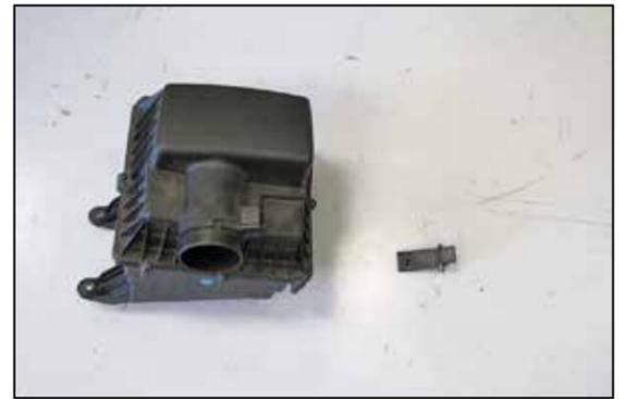
19. Remove the mass air sensor from the factory air filter housing.
