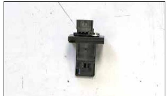
20. Install the mass air sensor into the K&N® mass air sensor adapter and secure with the provided hardware.
