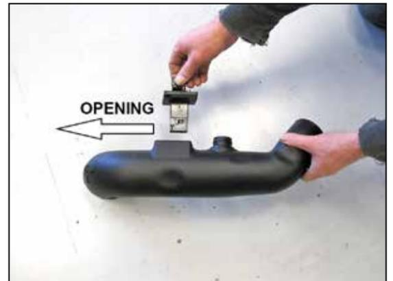
21. Install the mass air sensor assembly into the K&N® intake tube so that the opening is towards the filter.
