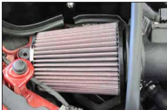
17. Install the air filter onto the K&N® intake tube and secure with the provided hose clamp. Adjust the tube and heat shield for best fit and then secure them with the hose clamp and hardware.
