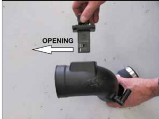
15. Install the mass air sensor assembly into the K&N® intake tube so that the opening in the sensor is towards the air filter end of the intake tube.
