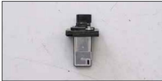
14. Install the mass air sensor into the K&N® mass air sensor adapter and secure with the provided hardware.
