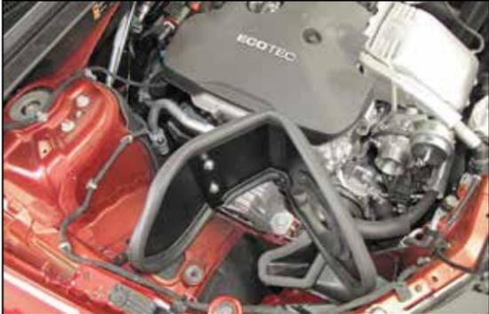
9. Install the heat shield assembly onto the engine mount and secure with the factory bolt from the previous step.
