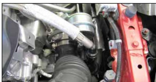
3. Disconnect the crank case vent hose.
