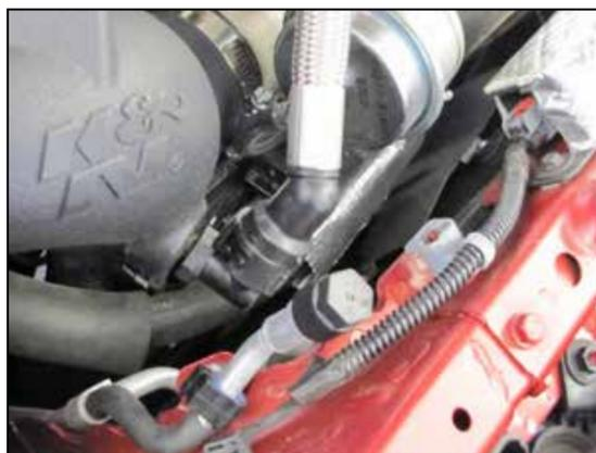
18. Connect the crank case vent hose to the fitting installed into the K&N® intake tube.
