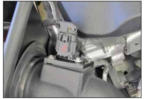
19. Reconnect the mass air sensor electrical connection.
