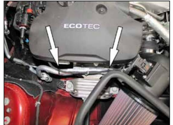
20. Using the provided tie wraps, secure the mass air sensor electrical cable to the A/C line as shown.
