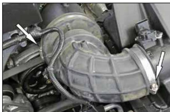
3. Loosen the two hose clamps that secure the intake tube to the turbo inlet and air filter housing. Remove the intake tube from the vehicle.
