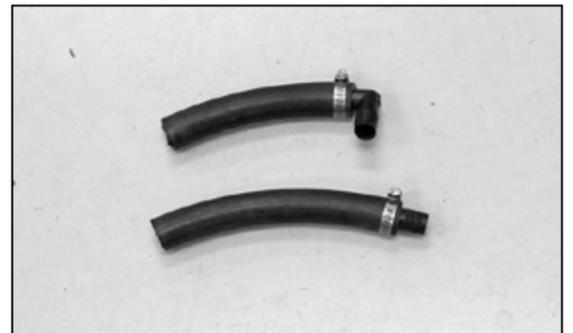
22. Install the provided union fittings into the vent hoses as shown and secure with the provided clamps. The 90° fitting will be installed into the 5" long hose.
