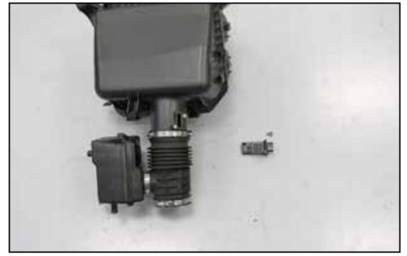
17. Remove the mass air sensor from the factory air filter housing.
