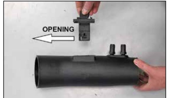
19. Install the mass air sensor assembly into the K&N® intake tube so that the opening in the sensor is towards the inlet end of the tube and then secure it with the provided hardware.
