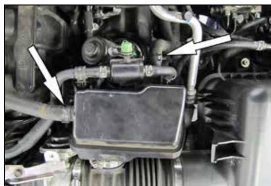
4. Release the spring clamps that secure the crank case breather hoses to the plenum chamber and then disconnect the crank case vent hoses. Unhook the EVAP canister from the plenum chamber.
