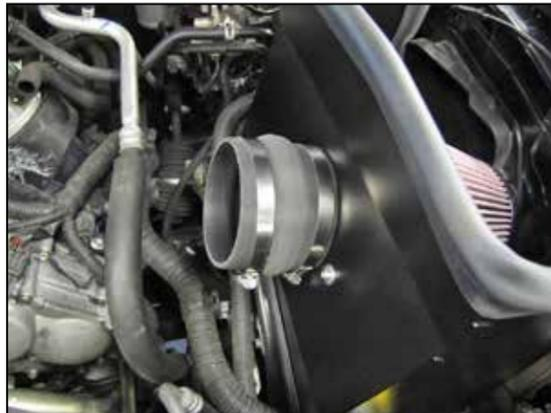
14. Install the provided hump coupler (08418) onto the filter adapter and secure with the provided hose clamp.
