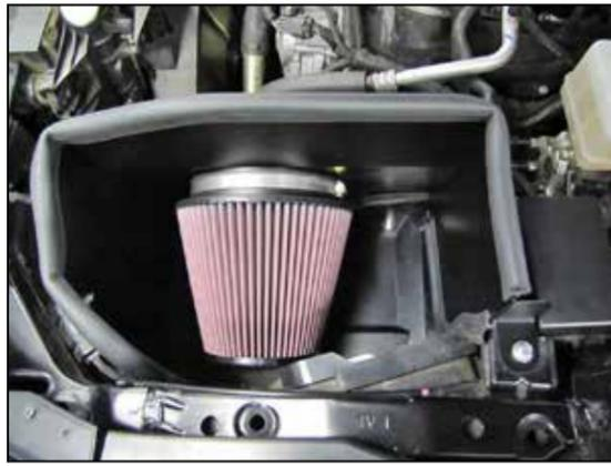
12. Install the heat shield assembly into the vehicle and secure it to the factory air filter housing mounting locations using the provided hardware.
