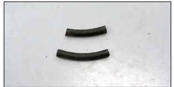
21. Cut the provided crank case vent hose into two sections, one section will be 5" long and the other will be 6-1/2" long.
