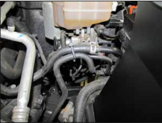
25. On 4 wheel drive vehicles, using one of the provided tie wraps secure the front differential breather to the EVAP lines.
