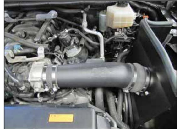
20. Install the K&N® intake tube into the hump coupler and then into the coupler at the throttle body, adjust the tube for best fit and then secure with the provided hose clamps.
