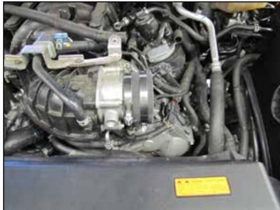
13. Install the provided coupler hose (08698) onto the throttle body and secure with the provided hose clamp.
