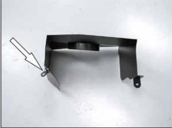
8. Install the mounting bracket (070066A) onto the heat shield using the provided hardware.
