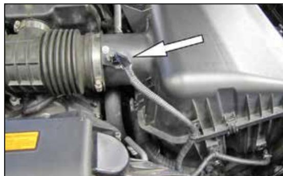
3. Disconnect the mass air sensor electrical connection and unhook the harness from the air filter housing.
