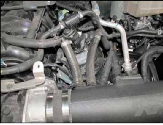
23. Install the vent hose assemblies into the factory vent hoses as shown; secure the factory vent hoses to the unions with the factory spring clamps. Connect the open ends of the hoses to the fittings installed into the K&N® intake tube.
