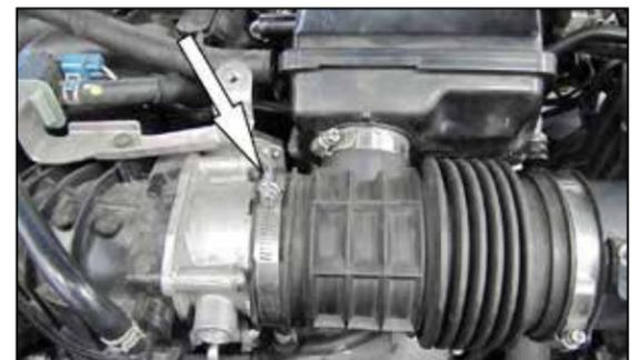
5. Loosen the hose clamp that secures the intake tube to the throttle body.
