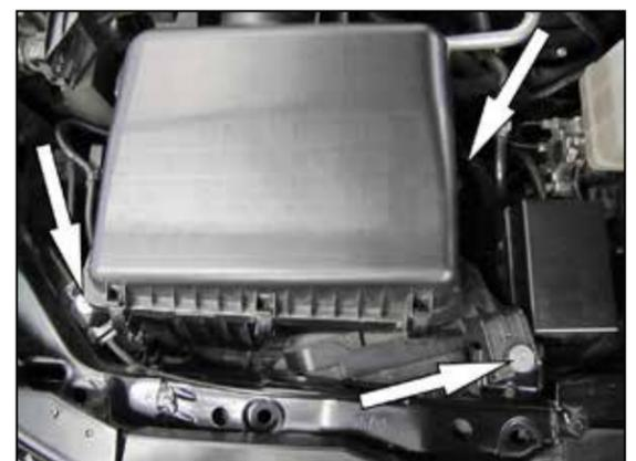
6. Remove the three bolts that secure the air filter housing to the inner fender and then remove the complete intake system from the vehicle.
