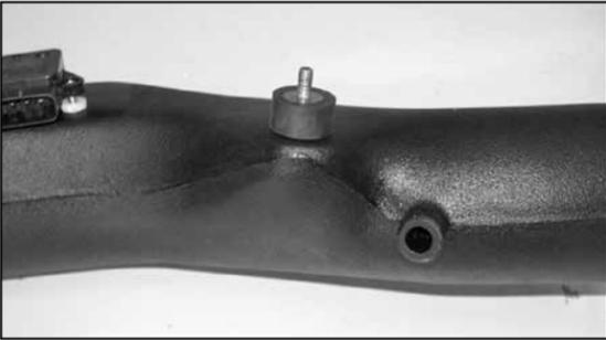
26. Install rubber mounted stud onto K&N® intake tube as shown.
