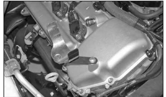
20. Install the saddle bracket assembly onto the threaded boss on the cam cover with the provided hardware as shown.
