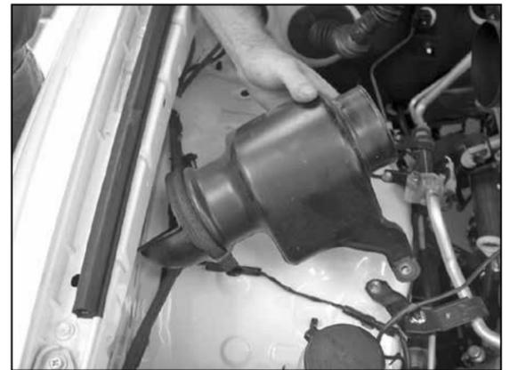
6. Remove two bolts that secure resonator to inner fender, then remove resonator from vehicle as shown.
