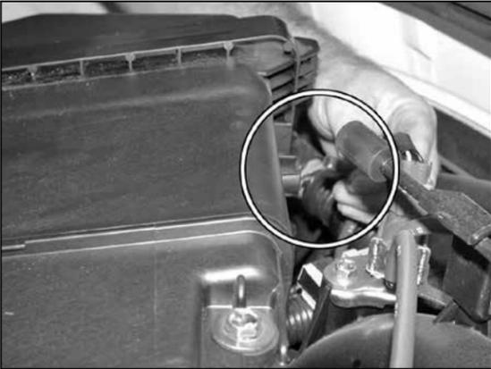
9. Remove fuel pressure regulator hose from back side of air box.
