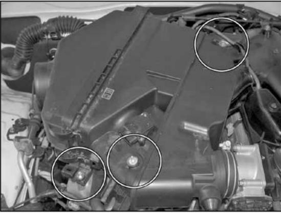
10. Loosen the hose clamp at throttle body, then remove the two bolts that secure air box to engine.
