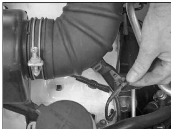
4. Pull wire harness clip up to release from intake tube.
