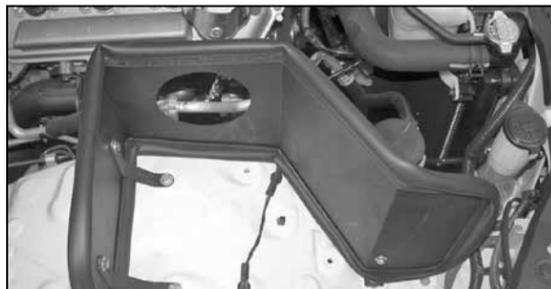
17. Install the heat shield onto the vehicle, then secure to brackets with the provided hardware.
