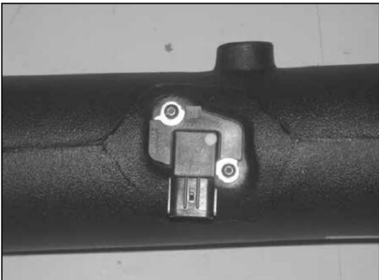
10. Install the mass air sensor into the K&N® intake tube and secure with the provided spacers and hardware as shown.
