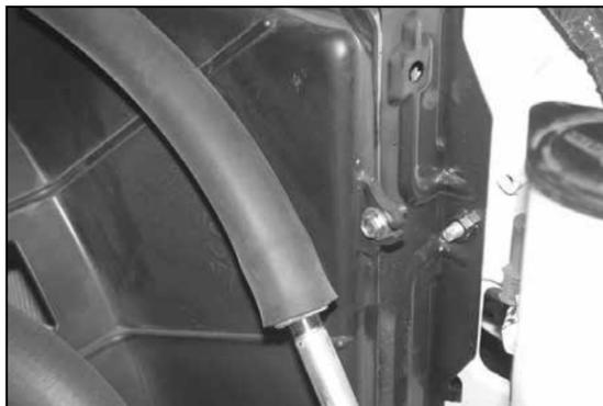
15. Remove the radiator fan shroud upper mounting bolt shown.
