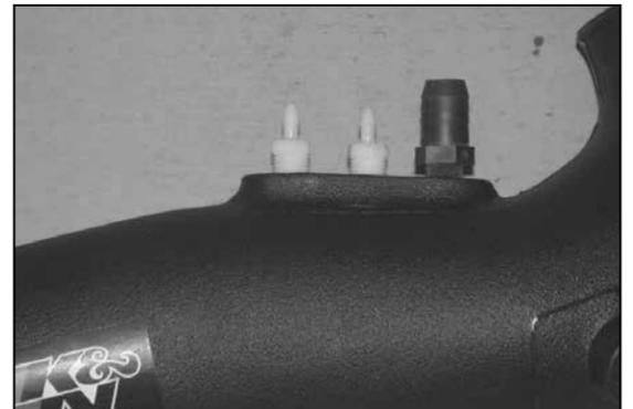
19. Install the provided npt fittings into the intake tube as shown.
