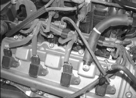
22. Remove the factory crankcase vent hose and fuel pressure regulator vent hose shown from the engine.
