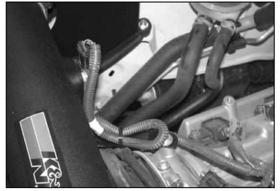
31. Using the provided wire tie, safely secure the excess mass air sensor wiring.
