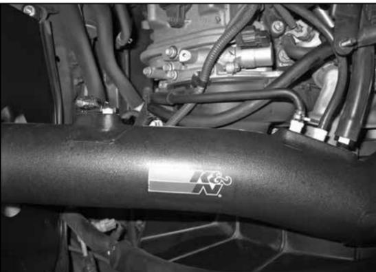
25. Attach the power steering pressure switch vent hose to the intake tube as shown.
