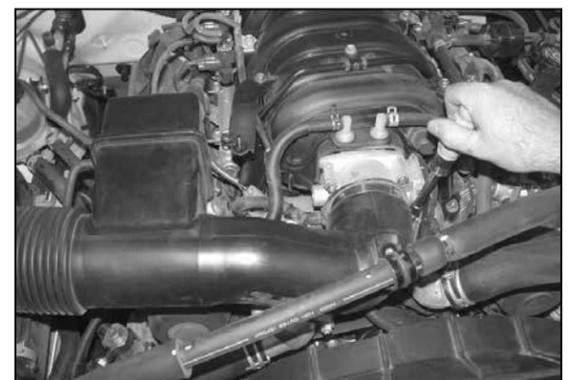
5. Loosen the hose clamp, which secures the stock intake tube to the throttle body
