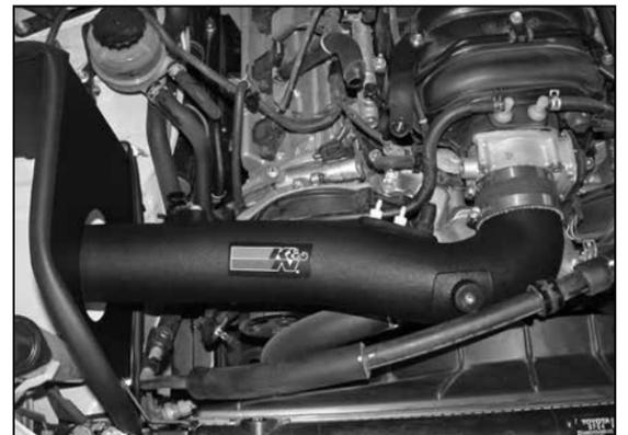
20. Install the intake tube onto the throttle body and align with the tube mounting bracket, Then secure with the provided hardware.
