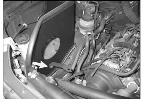
17a. Install the tube mounting bracket (083113) onto the heat shield a shown using the provided hardware.
