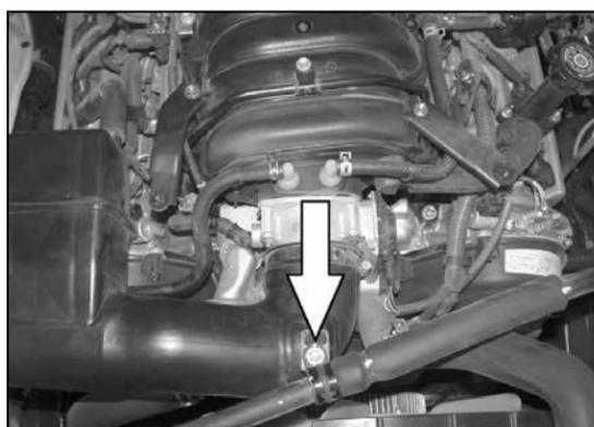
4. Loosen and remove the bolt that secures the A/C hose to the stock intake tube.
