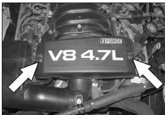
3. Loosen and remove the nuts shown that secure the throttle body cover, then remove the throttle body cover from the engine.
