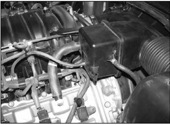
7. Disconnect the three vacuum lines shown from the stock intake tube.
