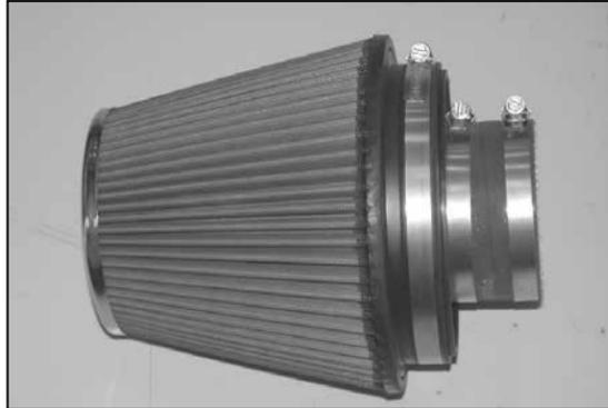
27. Install the silicone hose (08630) onto the filter adapter as shown and secure with the provided hose clamp.
