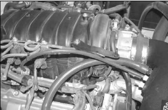
24. Install the provided fuel pressure regulator vent hose onto the fuel pressure regulator and then attach to the intake tube as shown.
