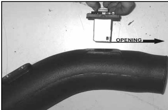
25. Install the mass air sensor assembly into the K&N® intake tube and secure with the provided hardware.
