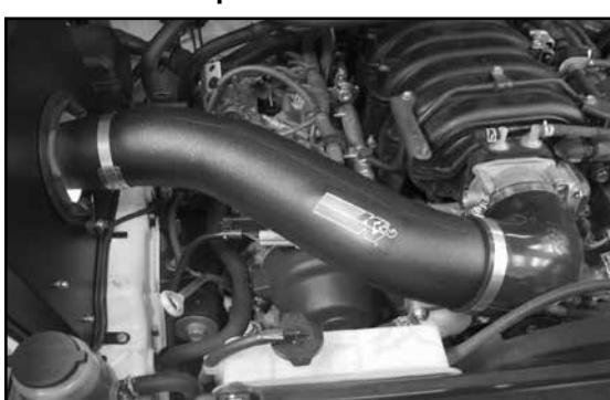
27. Install the K&N® intake tube into the silicone hose at the throttle body and align with the tube mounting bracket installed in step #11. Secure the intake tube with the provided hose clamps.
