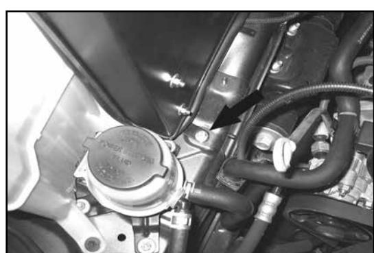
19. Secure the front heat shield bracket to the front air box location with the provided hardware.
