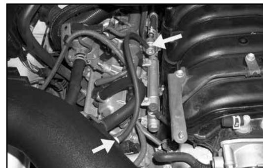
29. Install the provided fuel pressure hose onto the fuel pressure regulator, then connect the open end to the NPT fitting installed into the K&N® intake tube as shown.
