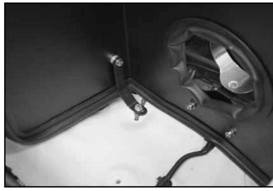
18. Set the heat shield into position on the inner fender. Secure the "C" bracket to the ground strap location.
