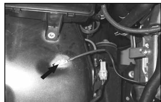
17. Remove the bolt that retains the ground strap to the inner fender.
