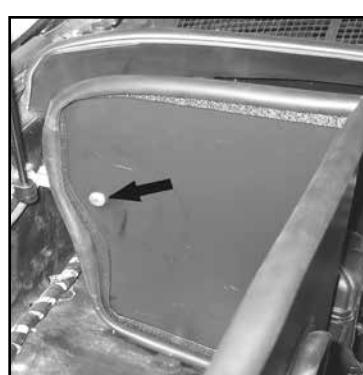
20. Secure the rear of the heat shield to the bracket installed in step #12.
