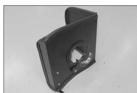
16. Install the tube mounting bracket assembly onto the heat shield as shown using the provided hardware.
