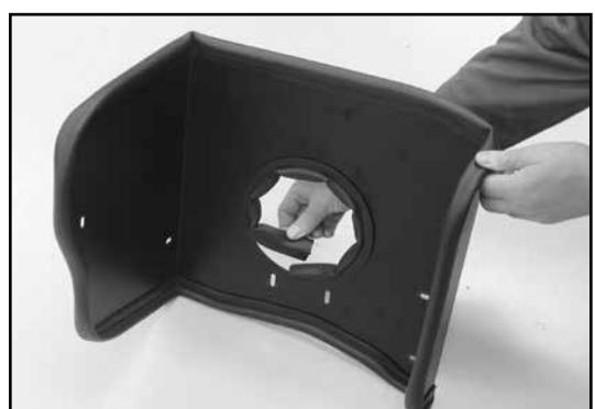
11. Install the short edge trim into the hole in the heat shield as shown.
