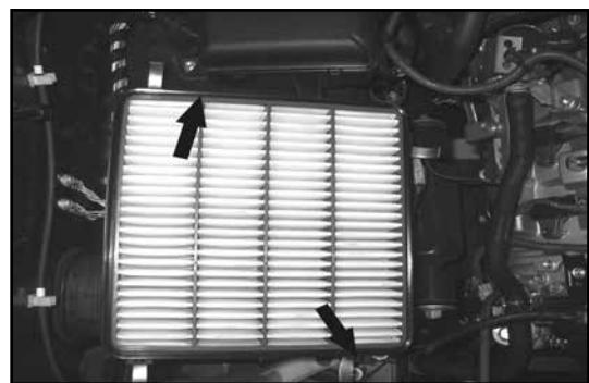
7. Remove the two factory bolts that secure the lower air box to the inner fender.
