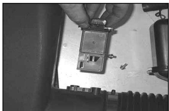
23. Remove the two factory screws that secure the mass air sensor, then remove the mass air sensor from the stock intake tube.
