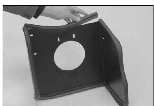
10. Install the long edge trim onto the heat shield as shown.
