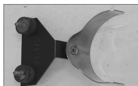
15. Install the saddle clamp onto the tube mounting bracket as shown using the provided hardware.
