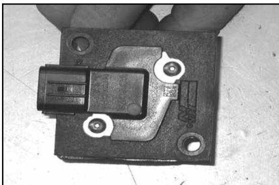
24. Install the mass air sensor into the K&N® mass air sensor adapter and secure with the provided hardware.
