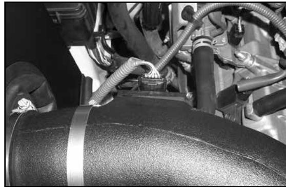
33. Re-connect the mass air sensor electrical connection.
