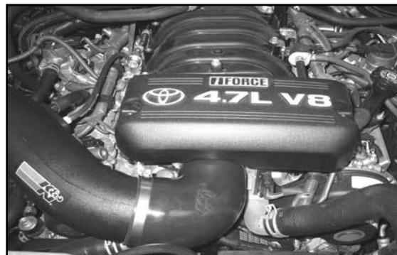
34. Re-install the engine cover and secure with the factory nuts.
