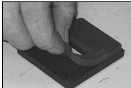
22. Install the provided gasket onto the K&N® mass air sensor adapter as shown.
