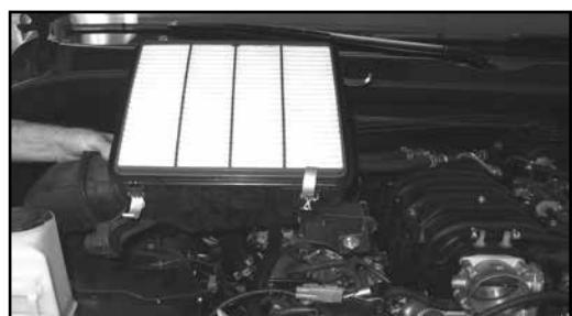
8. Lift the air box up, releasing it from the inner fender mounting grommet and fresh air duct. Remove the lower air box from the vehicle.
