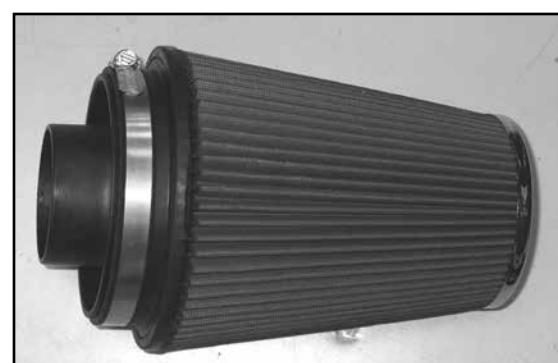
30. Install the provided air filter adapter into the K&N® air filter and secure with the provided hose clamp as shown.
