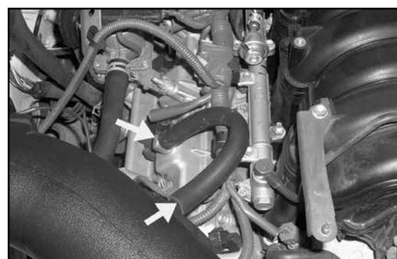
28. Install the provided crank case vent hose onto the valve cover fitting, then connect the open end to the NPT fitting installed into the K&N® intake tube as shown.
