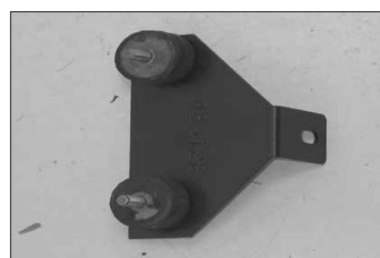
14. Secure the provided rubber mounted studs to the tube mounting bracket as shown using the provided hardware.
