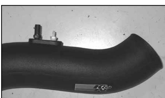
26. Install the provided 1/4" NPT fittings into the K&N® intake tube as shown.
