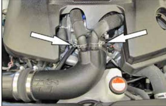
11. Install the crank case breather hoses and then secure with the factory spring clamps.
