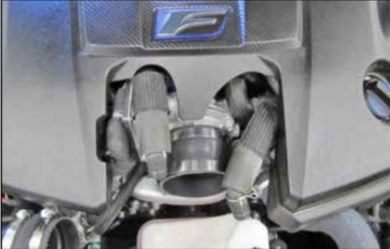
8. Install the coupling hose (084090) onto the throttle body and secure with the provided hose clamp.
