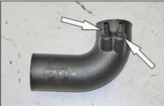
9. Install the provided vent fittings into the K&N® intake tube as shown.
