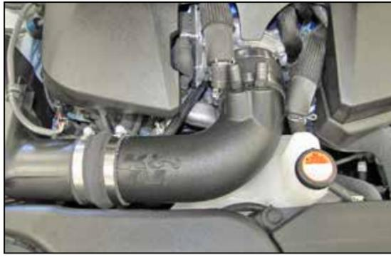
10. Install the K&N® intake tube assembly into the coupler at the air filter housing and then into the coupler at the throttle body. Adjust the tube for best fit and then secure with the provided hose clamps.
