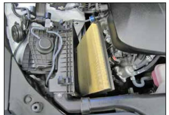
5. Place the housing up out of the way and remove the stock air filter from the lower housing.
