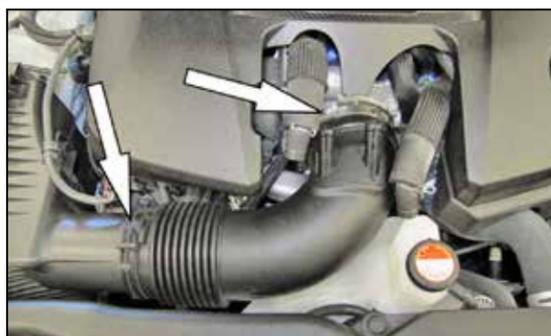
3. Loosen the hose clamps that secure the intake tube to the throttle body and air filter housing and then remove the intake tube from the vehicle.
