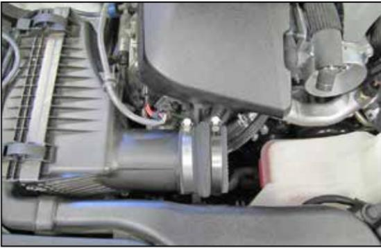
7. Install the coupling hose (08699) onto the air filter housing and secure with the provided hose clamp.
