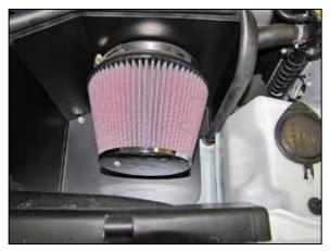
23. Install the K&N® air filter onto the filter adapter and secure with the provided hose clamp. NOTE: Drycharger® air filter wrap; part # 22-8049DK is available to purchase separately. To learn more about Drycharger® filter wraps or look up color availability please visit http://www.knfilters.com®.
