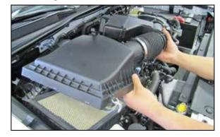
6. Release the two clips securing the upper air filter housing and then remove the intake tube and air filter hosing along with the factory air filter.
