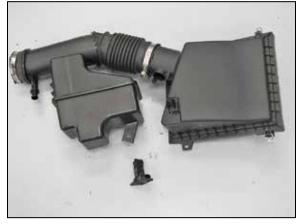
16. Remove the mass air sensor from the factory air filter housing.
