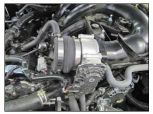
13. Install the provided coupler (08171) onto the throttle body and secure with the provided hose clamp.
