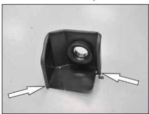
11. Install the provided edge trim onto the K&N® heat shield as shown.
