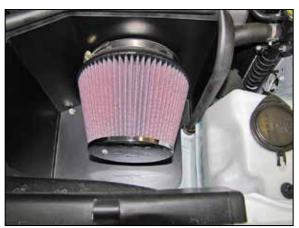
23. Install the K&N® air filter onto the filter adapter and secure with the provided hose clamp.
