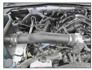
20. Install the intake tube into the coupling hose at the throttle body and then into the coupling at the filter adapter. Adjust the tube for best fit and then secure with the provided hose clamps.
