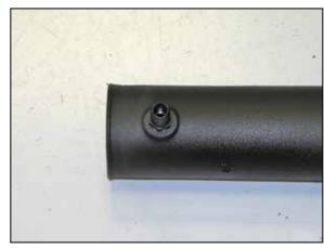
19. Install the provided NPT vent fitting into the  $K\&N^{\tiny \circledcirc}$  intake tube as shown.
