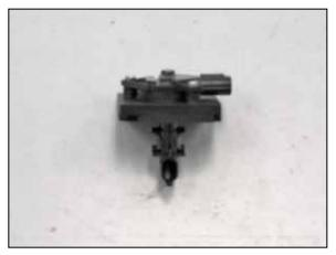
17. Install the mass air sensor into the adapter and secure with the provided hardware.
