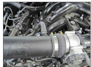
21. Connect the crank case vent fitting onto the vent fitting installed into the K&N® intake tube.
