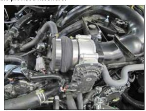
13. Install the provided coupler (08171) onto the throttle body and secure with the provided hose clamp.
