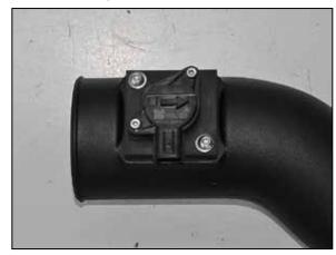
18. Install the mass air sensor assembly into the K&N® intake tube and secure with the provided hardware.
