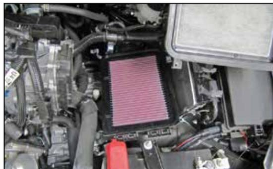
4. Release the clips that secure the upper air filter housing, lift up the housing and remove the factory air filter. Install the provided K&N® air filter and then reinstall the upper housing and secure with the factory retaining clips.
