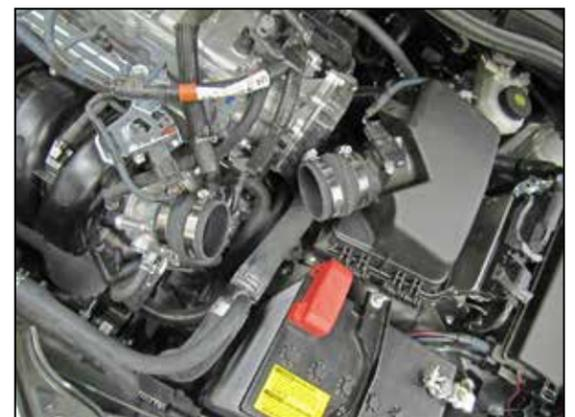
5. Install the provided hump couplers onto the throttle body and air filter housing and secure with the provided hose clamps.
