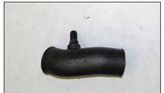
6. Install the provided crank case vent fitting into the K&N® intake tube as shown.
