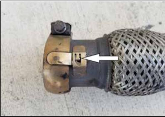
8. Once stock system is removed, remove the conical clamp by prying retaining tang upwards.
