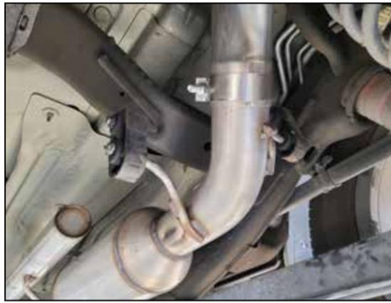
11. Slide band clamp on to the front of the tail pipe section. Then slide tail pipe section into muffler section. **NOTE:** Do not tighten the tail pipe connection at this time. Only enough to allow positioning of the tip to the body of the vehicle.
