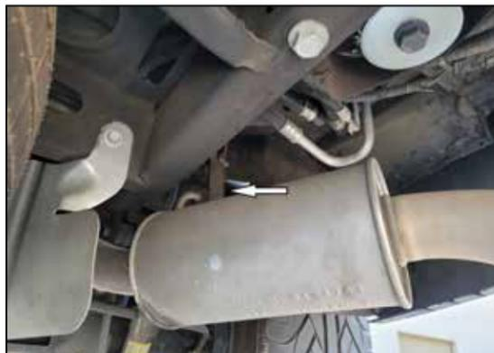
4. Remove rear tail pipe section by sliding tail pipe off rear hanger (leave rubber hanger on vehicle).
