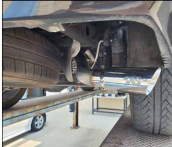
12. Check alignment and reposition as necessary. Once final position is satisfactory, tighten all hardware and band clamps from front to rear of vehicle. Clean exhaust tip of any finger prints or grease marks. **NOTE: All band clamps should be torqued to 40-45 ft-lbs.**
