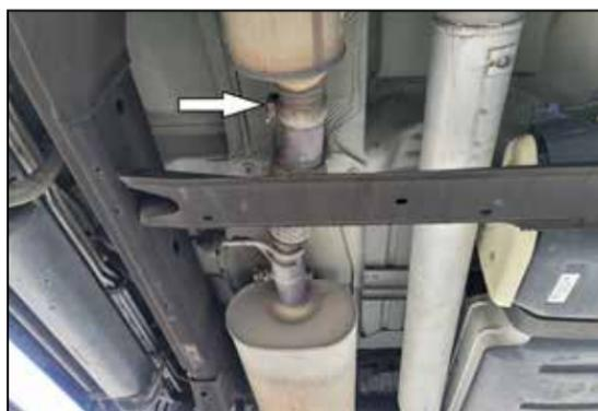
5. Once rear tail pipe has been removed loosen front conical clamp connecting tail pipe to head pipe.
