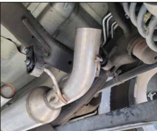
10. Slide mid pipe muffer assembly into position on the vehicle by first using the hangers on the muffler end. Once inserted, then slide assembly rearward allowing the mid pipe to seat against head pipe.
