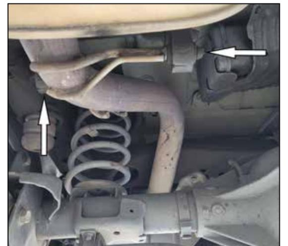
6. Remove muffer assembly from remaining hangers starting with the front hanger.
