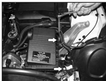
7. Models between April 2001-2004: Remove the two bolts that secure the air cleaner assembly as shown.
