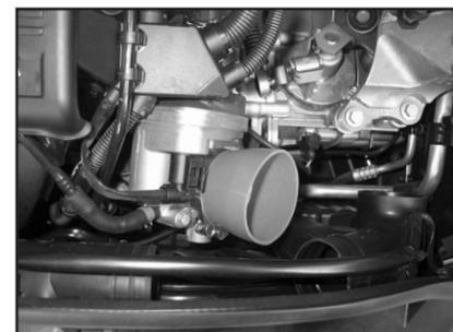
11. Secure the silicone stepped hose and hose clamps onto the throttle body as shown.
