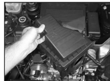
9. Remove the air cleaner assembly from the vehicle as shown.
