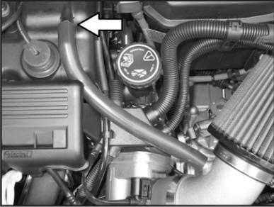
14. Install the provided silicone hose onto the crankcase vent on the cam cover, then, attach the other end onto the vent on the intake tube as shown.
