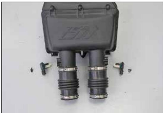
17. Remove the two mass air sensors from the factory air box.
