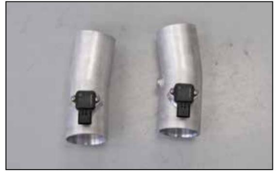
19. Install the mass air sensors into the K&N® intake tubes and secure with the provided hardware.
