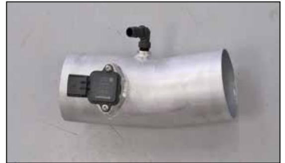
20. Install the provided 90° 1/4 npt vent fitting into the K&N® intake tube as shown.
