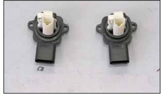
18. Remove the factory O-rings from the mass air sensor and then install the provided gaskets onto the sensors as shown.
