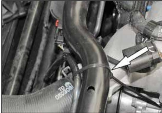
14. Secure the EVAP line to the frame cross member using the provided tie wrap.
