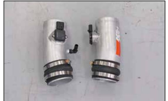
21. Install the provided hump hoses all the way onto the K&N® intake tubes as shown. Do not tighten at this time.
