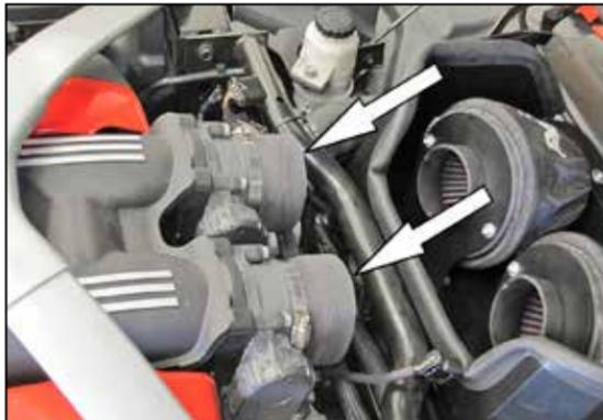
16. Install the two provided coupling hoses (08496) onto the throttle body and secure with the provided hose clamps.
