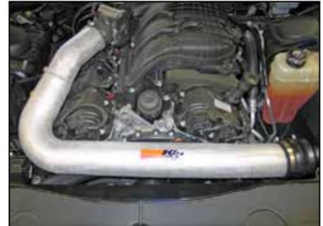
19. Install the K&N® intake tube into the silicone hump hose and then into the silicone hose on the throttle body.
