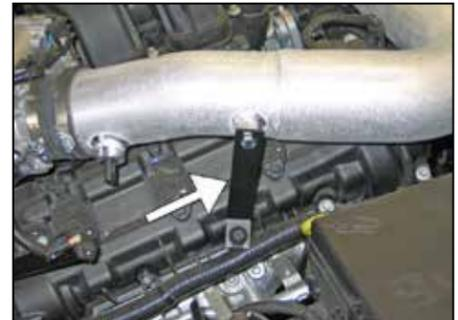
22. Install the tube bracket onto the mounting stud and then secure to the K&N® intake tube with the provided hardware. Tighten the hose clamps at this time.
