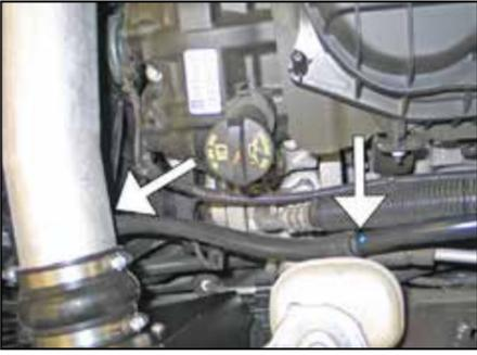
24. Install the provided silicone hose onto the factory crankcase vent tube and then connect the open end to the 90° fitting installed into the K&N® intake tube.
