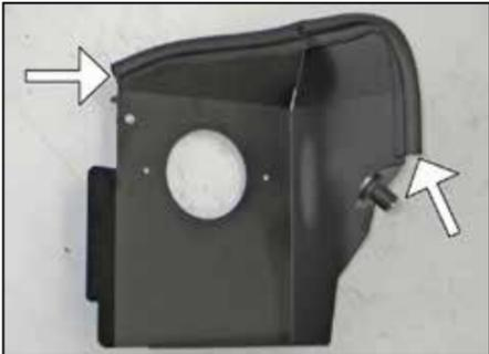
10. Install the provided longer edge trim onto the top of the heat shield as shown.
