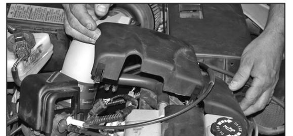
26. Reinstall the plastic coil cover as shown.
