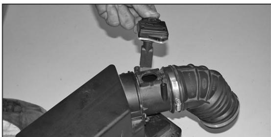
15. Remove the mass air sensor from the stock air cleaner assembly as shown using the provided Torx wrench.
