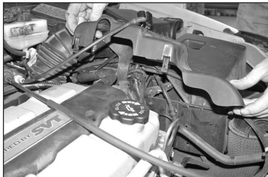
4. Pull up firmly to remove the plastic coil cover as shown.
