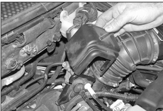
3. Pull up firmly to remove the plastic throttle linkage cover as shown.
