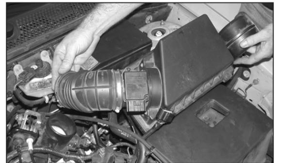
7. Pull firmly upwards to remove the air cleaner assembly as shown.
