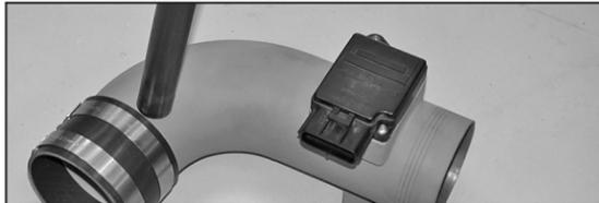
18. Install the mass air sensor into the tube and secure with the provided hardware as shown.
