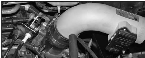
19. Install the tube into the vehicle and onto the throttle body as shown.
