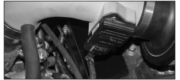
24. Reconnect the mass air sensor electrical connection as shown.
