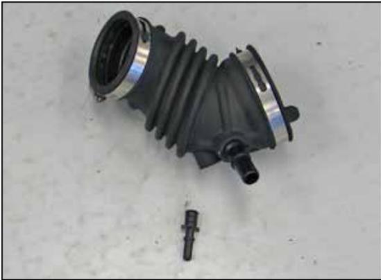
29. Remove the EVAP fitting from the intake hose.
