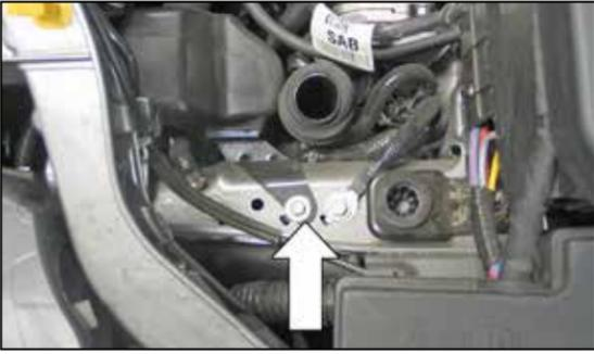
10. Remove the bolt shown securing the intake silencer to the inner fender; lift up to remove the intake silencer from the vehicle.
