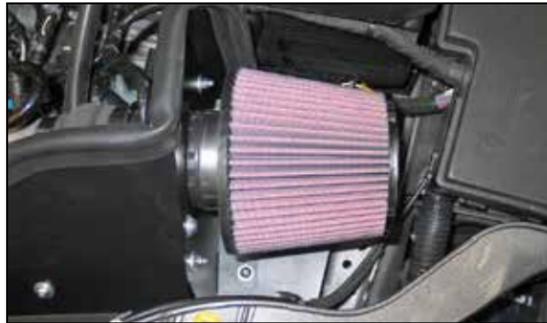
36. Install the K&N® air filter and secure with the provided hose clamp.
