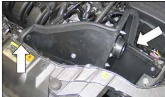
35. Install the 30" long section of edge trim onto the fresh air plate and heat shield as shown. Some trimming of the edge trim will be necessary.
