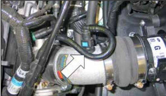
30. Install the EVAP fitting into the intake tube and then connect the EVAP vent line.
