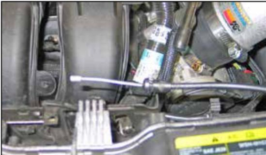
32. Disconnect the hood release cable from the hood latch.
