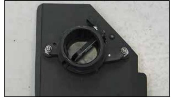
22. Secure the mass air sensor housing to the rubber mounted studs on the heat shield as shown using the provided hardware.
