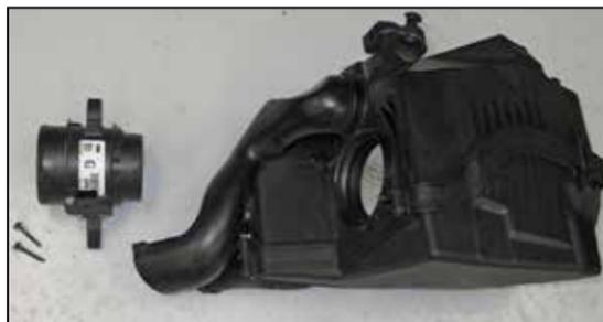
21. Remove the two bolts securing the mass air sensor housing to the air box; separate the mass air housing from the air box.
