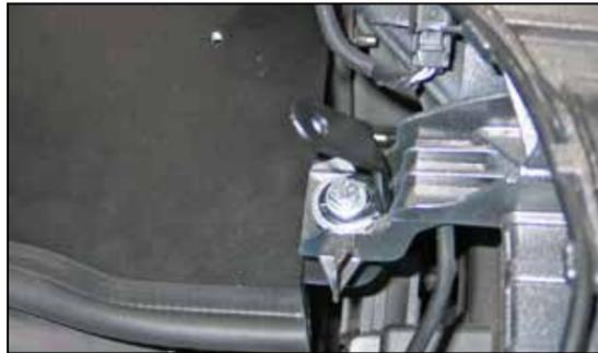
18. Using the provided hardware, secure the provided bracket (083161) to the fresh air intake scoop mount and the rubber mounted stud on the heat shield base.
