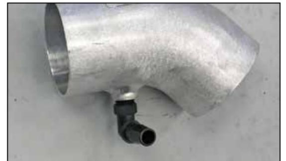
25. Install the 90° vent fitting into the K&N® intake tube as shown.
