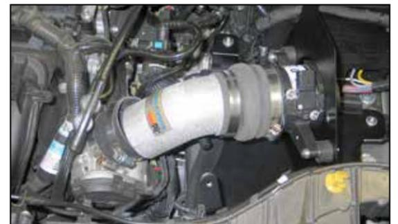
26. Install the K&N® intake tube completely into the silicone hump hose and then set the complete assembly onto the heat shield base.
