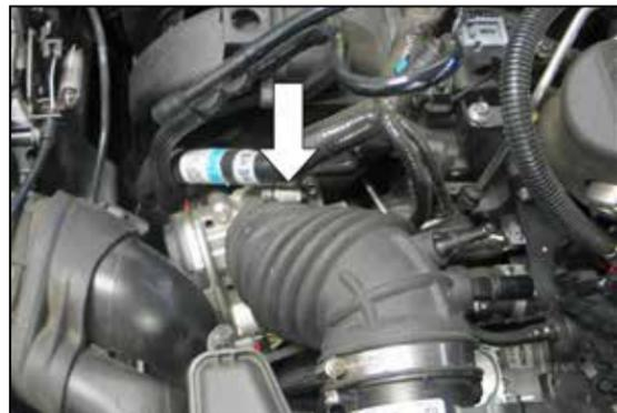
6. Loosen the hose clamp securing the intake tube to the throttle body.
