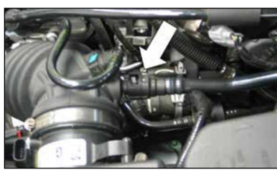
4. Disconnect the crank case vent line from the intake tube.
