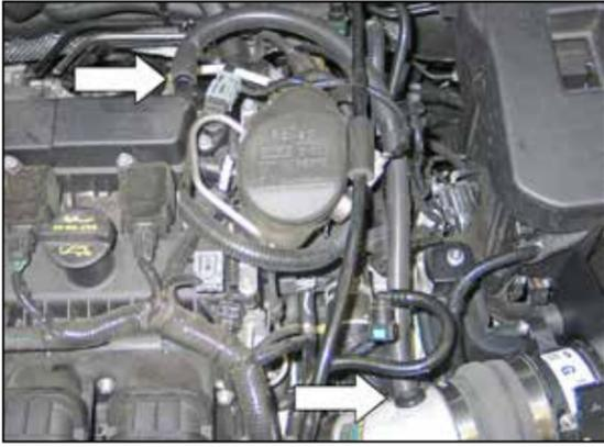
28. Install the provided silicone vent hose onto the 90° vent fitting in the K&N® intake tube and attach the open end to the valve cover port as shown.
