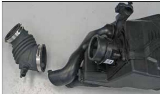
20. Loosen the hose clamp that secures the factory intake tube to the mass air sensor housing and then remove the hose from the mass air housing.
