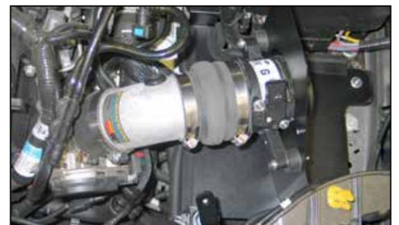
27. Install the K&N® intake tube into the silicone hump hose on the throttle body, then align the heat shield and secure with the provided hardware. Align the intake tube and secure with the provided hose clamps.
