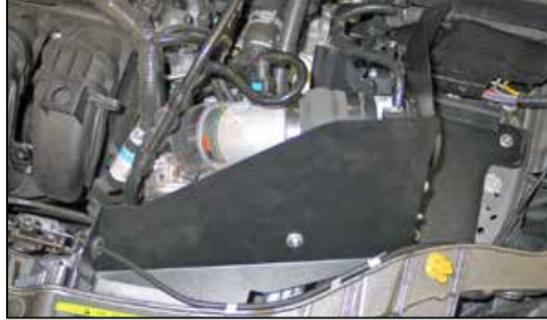
34. Pass the hood release cable through the grommet installed into the K&N® fresh air plate and then secure the fresh air plate to the heat shield and mounting bracket with the provided hardware. Reinstall the hood release cable to the hood latch.
