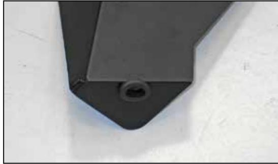
33. Install the provided 7/8"OD grommet into the K&N® fresh air plate as shown.
