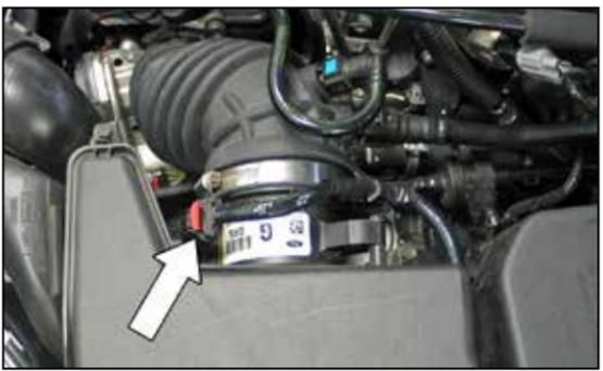
2. Release the red locking tab and then disconnect the mass air sensor electrical connection. Also unhook the mass air sensor wiring harness clip from the mass air sensor.
