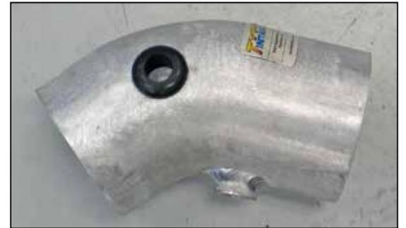
24. Install the provided 1.0"OD grommet into the K&N® intake tube as shown.
