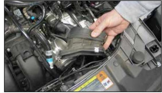
9. Remove the rubber fresh air duct from the vehicle.
