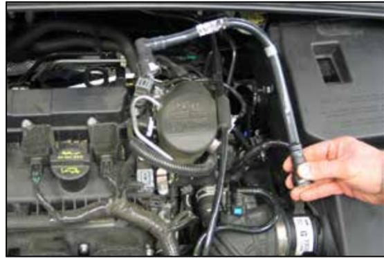
5. Disconnect the crank case vent hose from the valve cover and then remove the vent hose from the vehicle.
