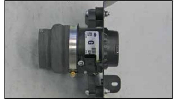
23. Install the provided hump hose (08421) onto the mass air sensor as shown and secure with the provided hose clamp.
