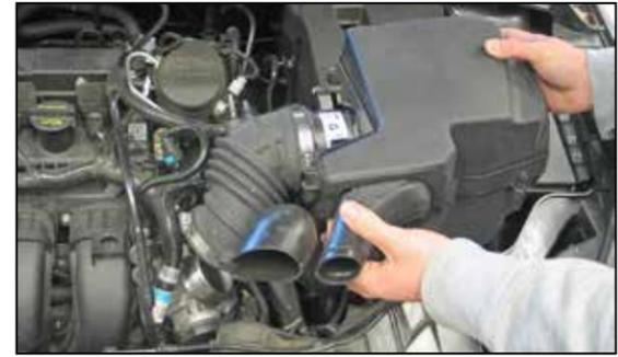
8. Lift up the air box assembly to release it from the mounting grommets; remove the air box from the vehicle.
