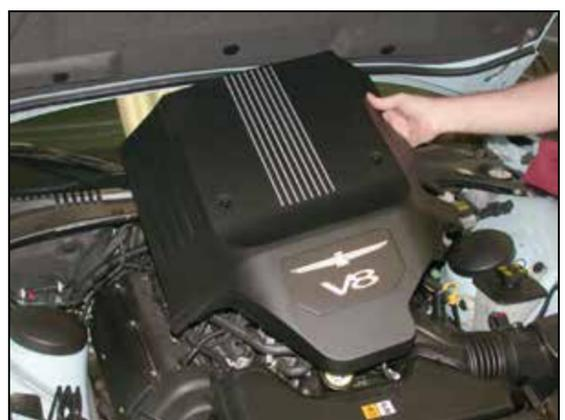
3. Pull up on the rear of the engine cover to dislodge from the retaining mounts, and then remove the engine cover from the engine.
