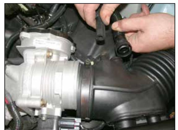
5. Disconnect the hoses from the stock intake tube as shown.
