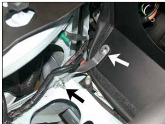
14. Install the provided heat shield bracket (010084) onto the bolt installed in step #14, and then fasten the bracket to the heat shield with the provided hardware.
