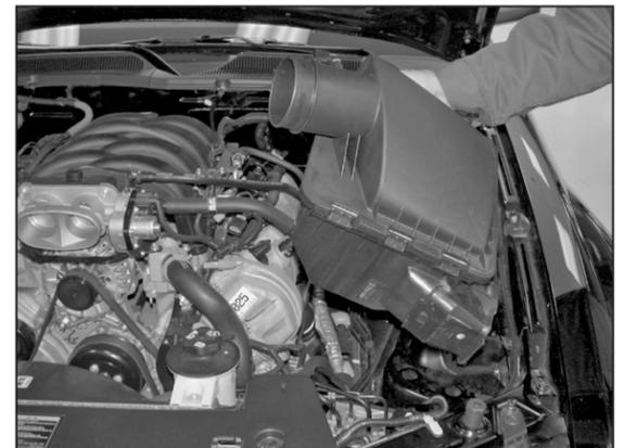
6. Remove the airbox assembly as shown. **NOTE: K&N Engineering, Inc., recommends that customers do not discard factory air intake.**
