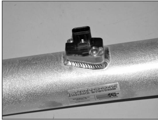
15. Install the mass air sensor into the K&N intake tube with the factory mounting screws.
