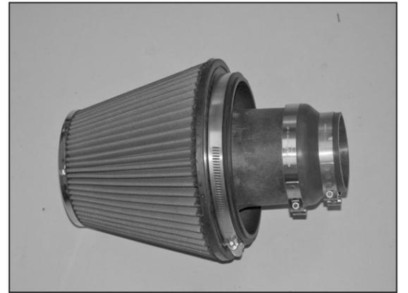
21. Install the silicone hose onto the air filter assembly and secure with the provided hose clamp as shown.
