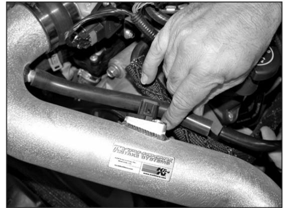
19. Install the provided crankcase vent hose onto the K&N intake tube and factory vent hose as shown.
