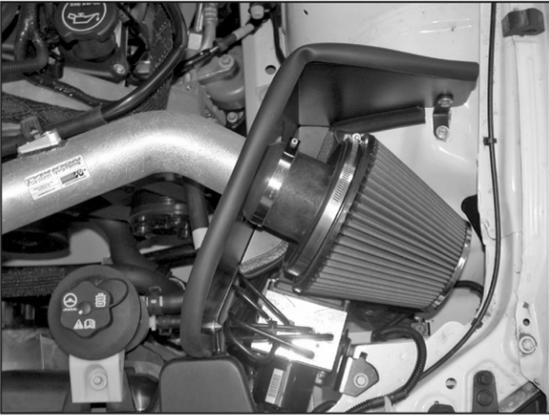
22. Install the K&N® air filter assembly onto the K&N® intake tube as shown and secure with the provided hose clamp.
