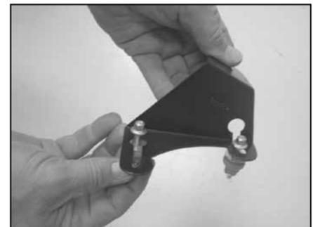
8. Install the valve cover bolts removed in step #7 into the tube mounting bracket as shown passing through the key hole portion and then slide the bolts to the end of the slots.
