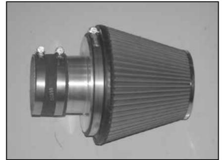
25. Install the air filter onto the filter adapter and secure with the provided hose clamp as shown.
