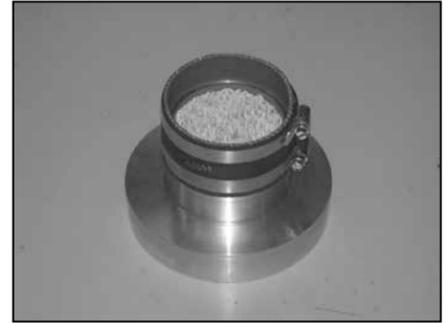
24. Install the silicone hose (08698) onto the filter adapter and secure with the provided hose clamp as shown.
