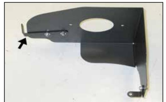
8. Install the large bracket (083129) onto the heat shield as shown and secure with the provided hardware.
