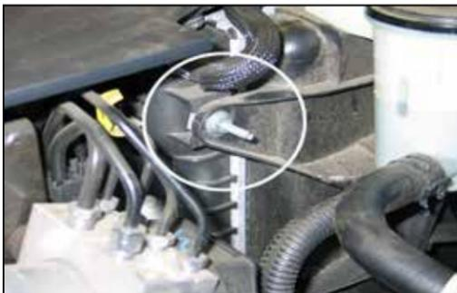
13. Remove the Left upper fan shroud mounting bolt shown.
