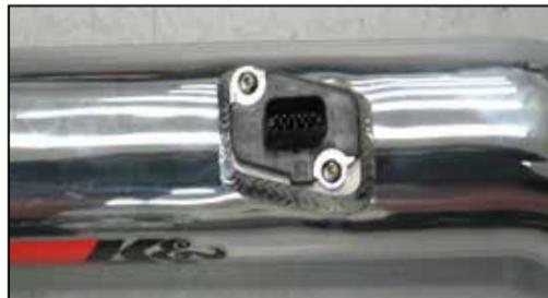
18. Install the mass air sensor into the K&N® intake tube and secure with the provided hardware.
