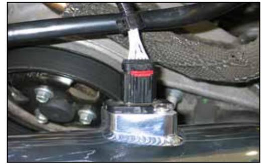
22. Install the K&N® mass air sensor harness extension into the factory wiring harness and then connect the open end into the mass air sensor.
