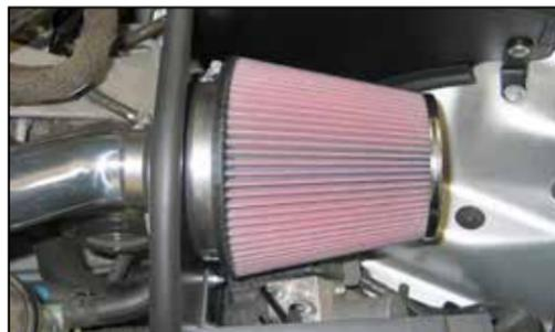
21. Install the K&N® air filter and secure with the provided hose clamp.
