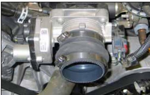
15. Install the provided hump hose (08421) onto the throttle body and secure with the provided hose clamp.
