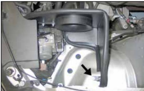
14. Set the heat shield into position on the inner fender and then secure to the inner fender and fan shroud with the hardware provided.
