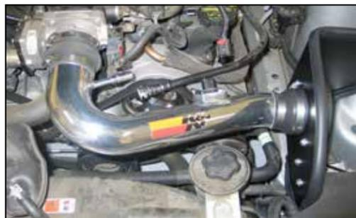
19. Install the K&N® intake tube into the silicone hose on the filter adapter and then into the silicone hose at the throttle body. Secure the intake tube with the provided hose clamps.
