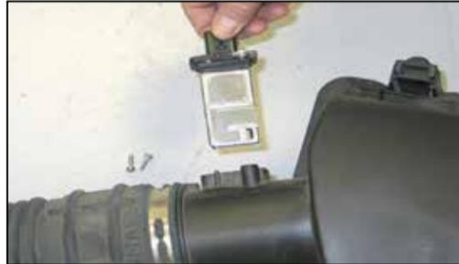
17. Remove the two screws which secure the mass air sensor and then remove the mass air sensor from the stock air box.
