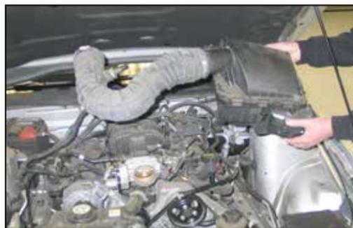
6. Remove the air box assembly from the vehicle.
