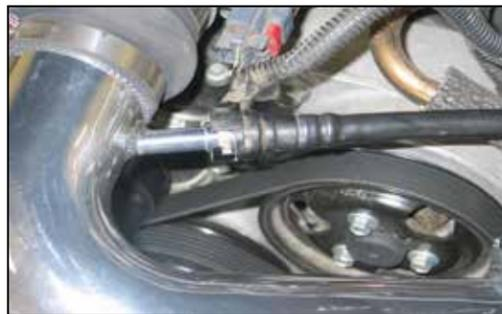
20. Connect the crank case vent hose to the K&N® intake tube as shown.
