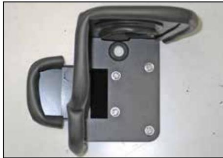
17. Attach the fresh air scoop to the heat shield using the provided hardware.
