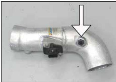
27. Install the provided 3/8" NPT vent fitting into the K&N® intake tube as shown.
