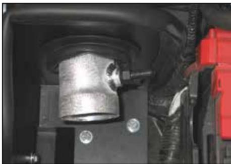
28. When equipped with EVAP, pass the K&N® intake tube through the heat shield and rotate so the remaining 1/2" npt vent fitting can be installed as shown.
