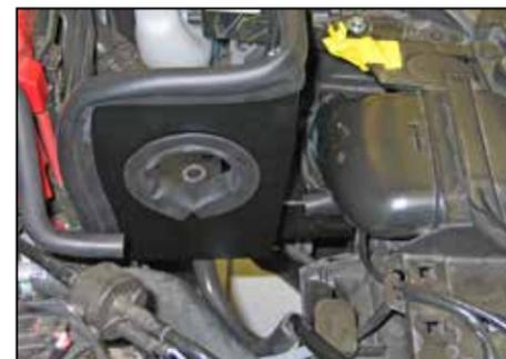
24. Install the fresh air scoop into the scoop attached to the heat shield and then reattach to the factory connection on the core support.
