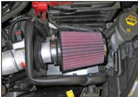
32. Install the K&N® air filter and secure with the provided hose clamp.
