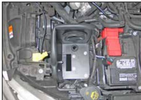
18. Install the heat shield assembly onto the vehicle so that the mounting studs are inserted into the factory mounting grommets, and then secure to the mounting bracket installed during step #10 with the provided hardware.
