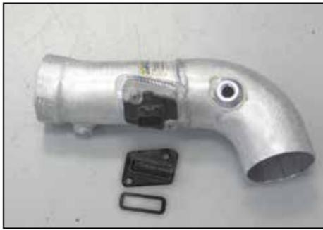
26. On vehicles that are equipped with a mass air sensor install the sensor into the K&N® intake tube and secure with the provided hardware. On all other vehicles, install the provided gasket onto the block off plate and install the block off plate into the K&N® intake tube and secure with the provided hardware.
