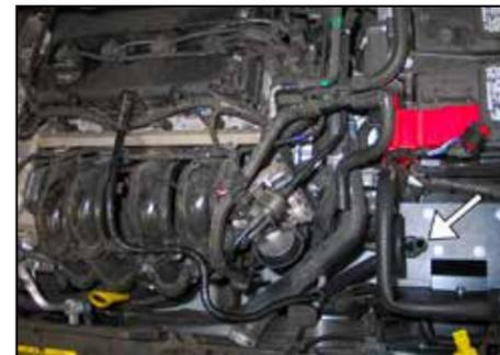
22. **US Models Only:** Reinstall the crankcase vent hose assembly onto the valve cover and route the silicone hose through the grommet in the bottom of the heat shield.
