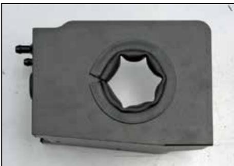
14. Install the 10" section of edge trim into the hole of the heat shield as shown.
