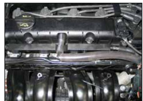
22a. **Non US models:** Install the provided 1/2" silicone vent hose onto the 1/4" vent and guide it along the fuel line towards the intake tube.
