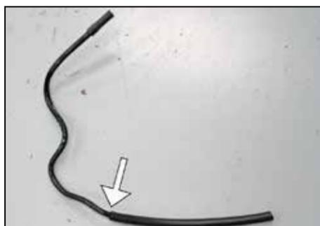
21. **US Models Only:** Install the provided 1/2" silicone vent hose onto the cut vent tube as shown.
