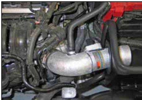
30. When equipped with EVAP, install the EVAP vent hose to the npt vent fitting.
