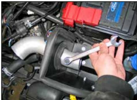
28a. Models without EVAP: Pass the K&N® intake tube through the heat shield and rotate so the provided NPT plug (08032) can be installed into the K&N® intake tube as shown.
