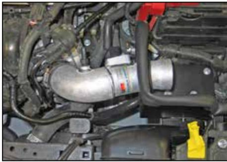
29. When equipped with EVAP, install the K&N® intake tube into the silicone hose at the throttle body and secure with the provided hose clamp. Attach the crankcase vent hose to the installed npt vent fitting.
