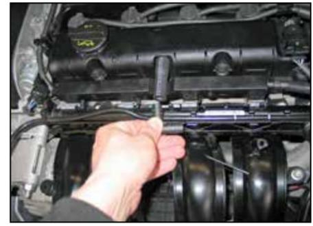
21a. Remove the rubber hose from the crankcase vent assembly and attach it to the valve cover as shown. Install the 1/4" 90° vent into the rubber hose as shown."
