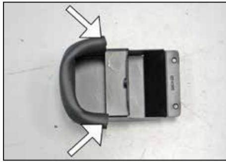
16. Install the 7" section of edge trim onto the fresh air intake scoop as shown.
