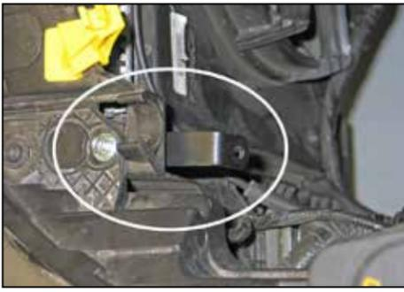
10. Install the heat shield mounting bracket (07195) onto the bottom of the bolt installed in the previous step along with the spacer provided.
