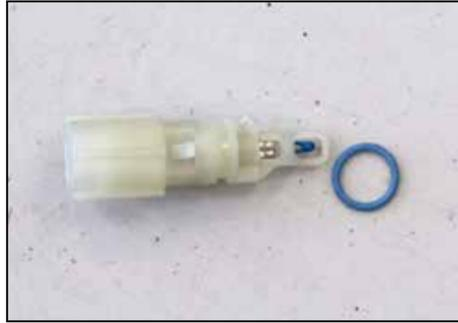
16a. Remove the grommet from the inlet air temperature sensor as shown.
