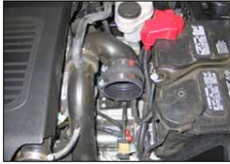
15. Install the provided silicone hump hose (08699) onto the factory inlet tube as shown and secure with the provided hose clamp.
