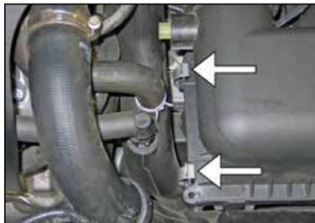
4. Release the two upper airbox retaining clips.
