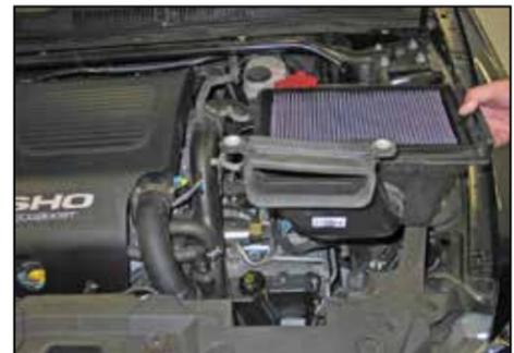
7. Lift up the airbox and remove it from the vehicle.
