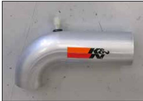
17. Install the provided grommet and the inlet air temperature sensor into the K&N® intake tube as shown.
