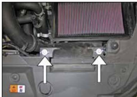
6. Remove the two bolts shown that secure the fresh air duct.
