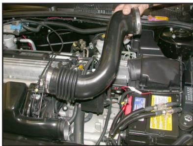
5. Loosen hose clamps and remove the stock intake tube as shown.
