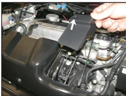
4. Disengage the plastic rivet and remove the throttle cable cover as shown.
