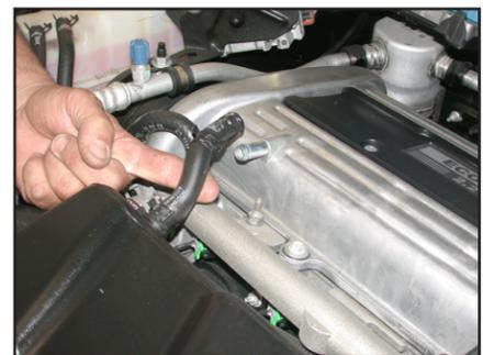
7. Remove the crankcase vent hose from the intake plenum as shown.
