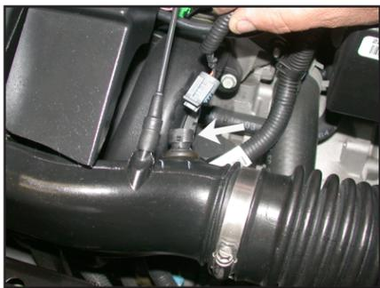
2. Disconnect the air temperature sensor electrical connection as shown.
