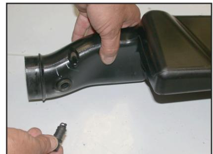
9. Remove the air temperature sensor from the intake tube as shown.
