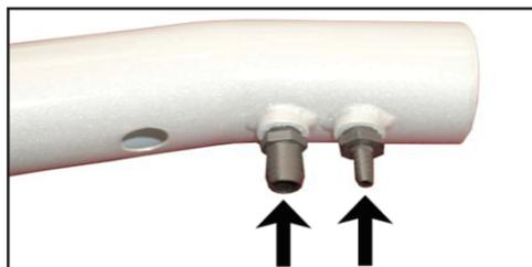
22. Install the two provided 1/4" NPT fittings into the K&N® intake tube as shown.
