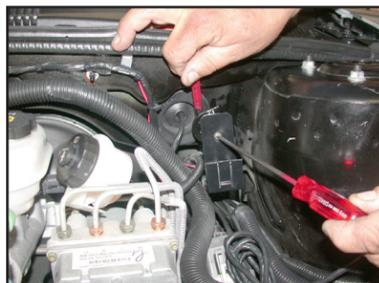
18. On manual transmission vehicles install the provided reservoir bracket onto the air cleaner locator bracket using the provided hardware as shown.
