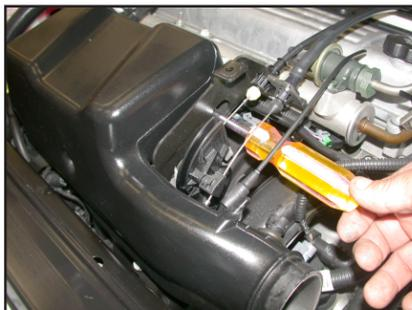
6. Loosen the hose clamp on the intake plenum at the throttle body as shown.
