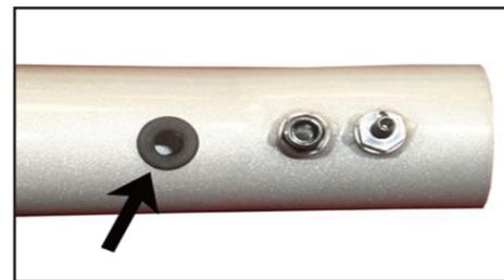
23. Install the provided grommet into the K&N® intake tube as shown.
