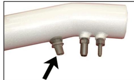
23a. Install the factory inlet air temperature sensor into the grommet installed into the K&N® intake tube in the previous step.
