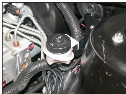
19. On manual transmission vehicles slide the fluid reservoir onto the bracket from step 18 as shown.
