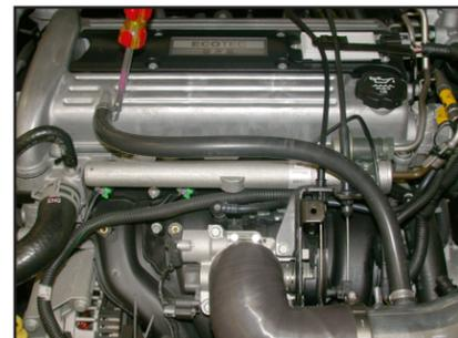
26. Connect the one end of the provided silicone hose to the vent on the cam cover, then, connect the other end to the vent on the K&N® intake tube and secure with the provided hose clamps as shown.
