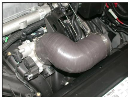
20. Install the silicone hose and hose clamps onto the throttle body as shown.
