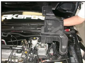
15. Rotate and pull the lower air cleaner assembly upwards to remove the assembly as shown.
