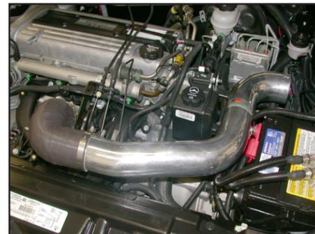
24. Install the K&N® intake tube into the silicone hose at the throttle body and align with the tube mounting bracket installed in step #21a. Secure the intake tube with the provided hose clamp and hardware.
