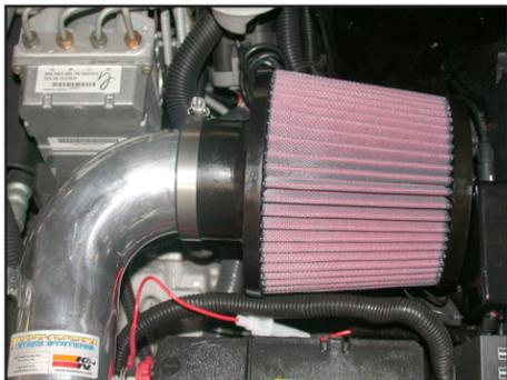
29. Install the K&N® air filter onto the K&N® intake tube and secure with the provided hose clamp as shown.
