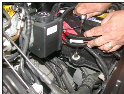
17. Reinstall the battery hold down block as shown.
