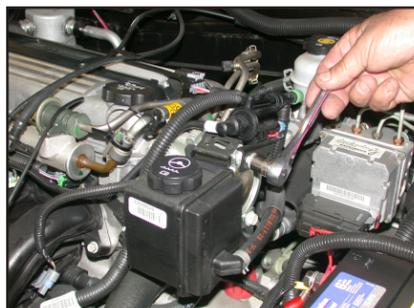
21. Remove the hex nut from the EVAP canister purge solenoid as shown.
