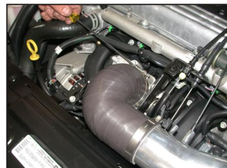
25. Adjust for best fit then tighten the hose clamps on the throttle body/intake tube as shown.
