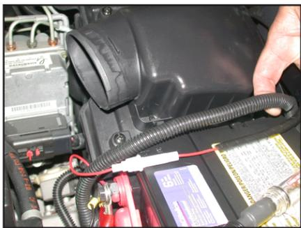
10. Unclip the wire harness from the air cleaner cover as shown.
