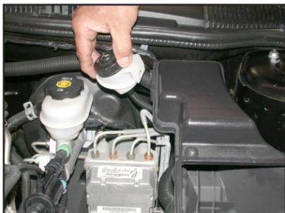
12. On manual transmission vehicles remove the fluid reservoir from the side of the lower air cleaner assembly as shown.
