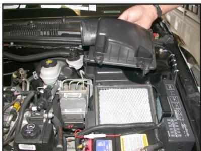
11. Loosen and remove the four air cleaner bolts to remove the air cleaner cover as shown.
