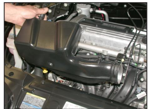
8. Pull upwards to remove the intake plenum as shown.
