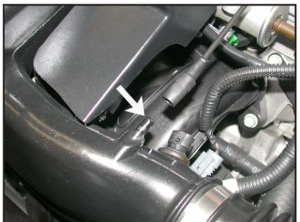
3. Disconnect the vent hose from the stock intake tube as shown.
