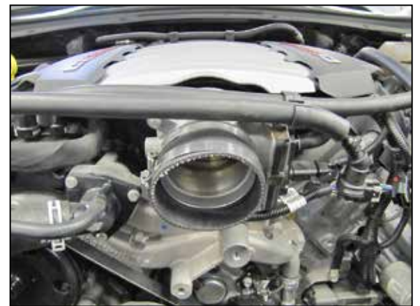
21. Install the provided coupler hose (08761) onto the throttle body and secure with the provided hose clamp.
