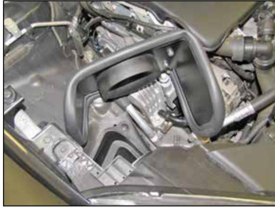
12. Using the factory bolt from the previous step, install the heat shield and spacer onto the motor mount as shown.
