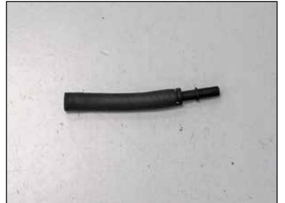
18. Install the provided quick disconnect union into the provided crank case breather hose.
