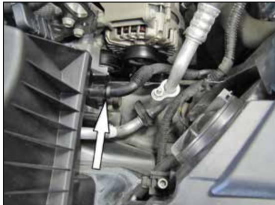
4. Disconnect the air filter housing drain.
