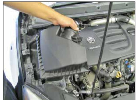
5. Lift up the air filter housing to dislodge it from the mounting grommets and then remove it from the vehicle.
