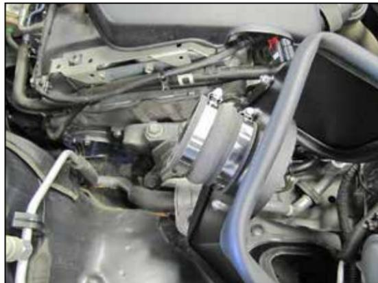
13. Install the provided coupler (087121) onto the filter adapter and secure with the provided hose clamp.
