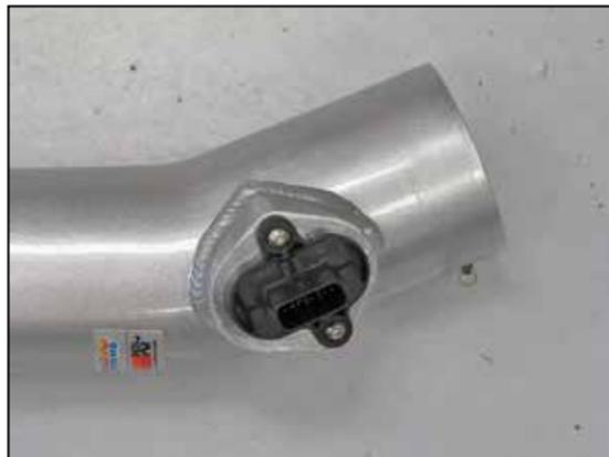
15. Install the mass air sensor into the K&N® intake tube and secure with the provided hardware.
