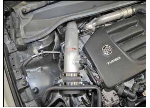
17. Install the K&N® intake tube into the turbo coupler and then into the filter adapter coupler. Adjust the tube and heat shield for best fit and then secure the hose clamps and heat shield hardware.
