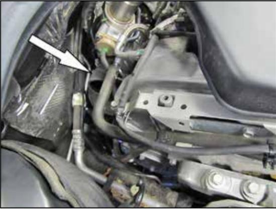
7. Install the provided coupling hose (084016) onto the turbo inlet and secure with the provided hose clamp.
