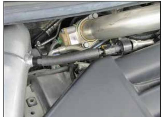
19. Install the crank case breather assembly into the factory quick disconnect fitting and then onto the vent fitting installed into the K&N® intake tube.
