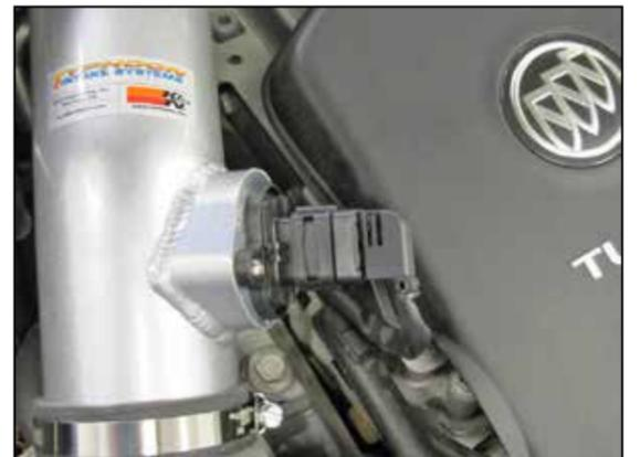
20. Reconnect the mass air sensor electrical connection.
