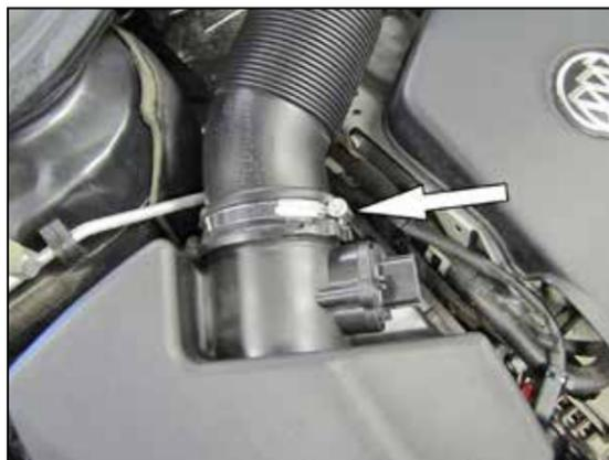
3. Loosen the hose clamp that secures the intake hose to the air filter housing.
