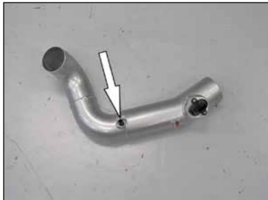
16. Install the provided vent fitting into the K&N® intake tube as shown.
