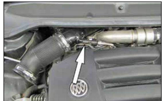
6. Disconnect the crank case vent quick disconnect fitting and then loosen the hose clamp that secures the intake tube to the turbo inlet. Remove the intake hose assembly.
