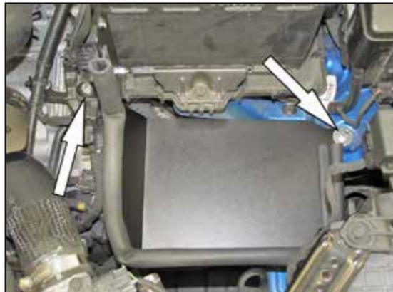
16. Install the heat shield onto the air filter housing mounting locations and secure with the provided hardware.
