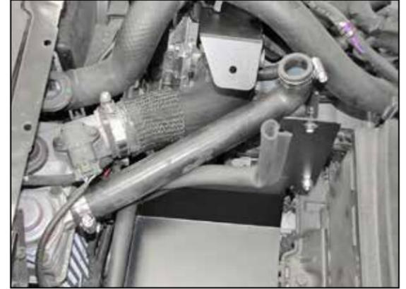
18. Install the provided BOV hose onto the BOV valve but do not tighten the hose clamp at this time.
