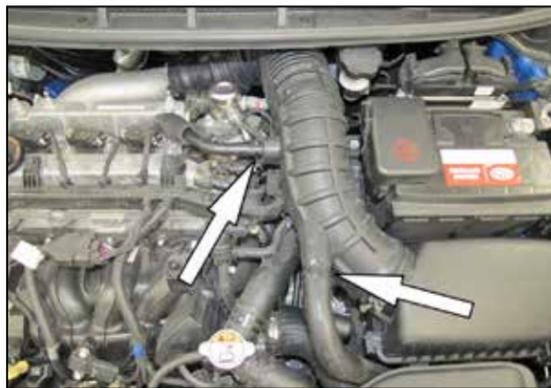
3. Release the spring clamps securing the crank case vent and BOV hose to the intake hose and disconnect the hoses from the intake hose.
