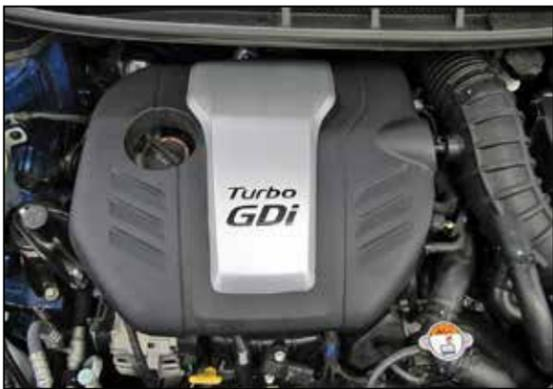
2. Lift up and remove the decorative engine cover from the vehicle.
