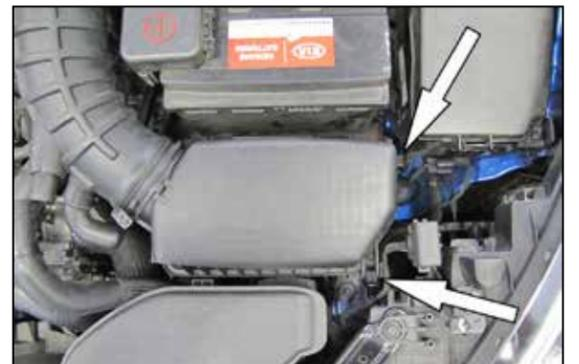
5. Release the two upper air filter housing retaining clips then lift up and remove the upper air filter housing and intake tube assembly.
