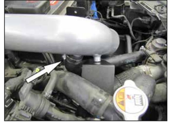
20. Connect the BOV hose to the K&N® intake tube and secure with the provided hose clamp.
