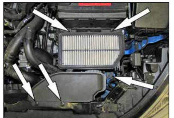
6. Release the two retaining clips securing the fresh air duct and then remove the three bolts securing the lower air filter housing and remove the lower air filter housing assembly.
