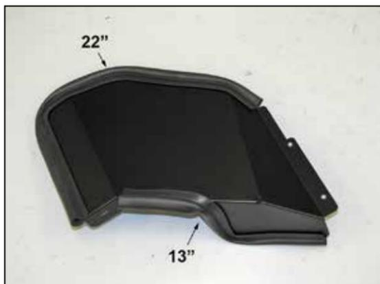
23. Install the remaining edge trim onto the heat shield as shown.
