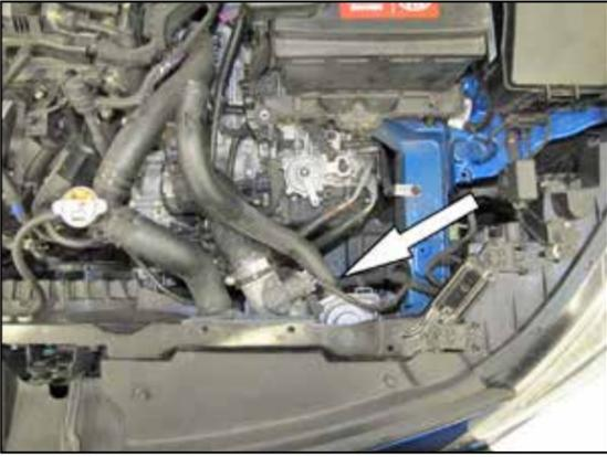
7. Release the spring clamp and then remove the BOV hose from BOV.
