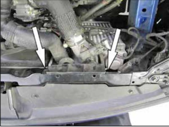
8. Remove the two bolts that secure the inner fresh air duct to the core support and then remove the inner fresh air duct.
