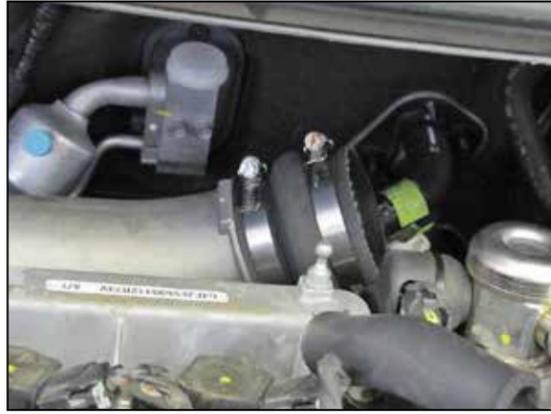
12. Install the provided coupling hose (08185) onto the turbo inlet tube and secure with the provided hose clamp.
