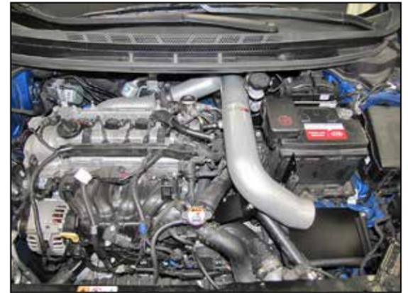
19. Install the K&N® intake tube into the coupler at the turbo inlet tube and align with the mounting bracket previously installed. Secure the tube with the hardware and hose clamp provided.
