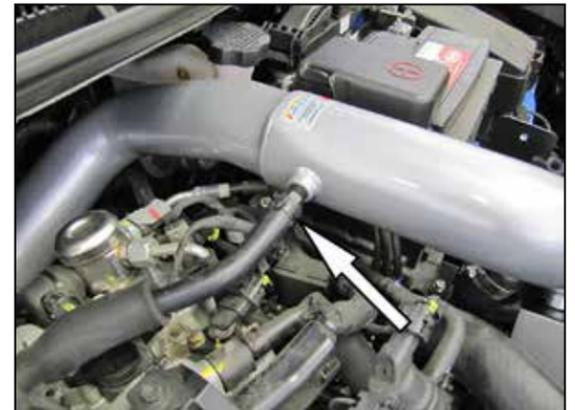
21. Connect the crank case vent hose to the K&N® intake tube and secure with the factory hose clamp.
