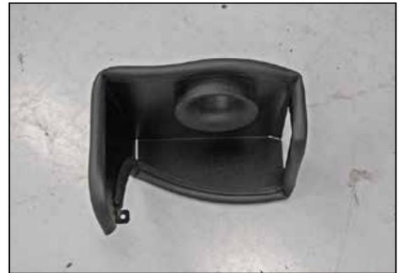
19. Install the edge trim onto the passenger side heat shield as shown.
