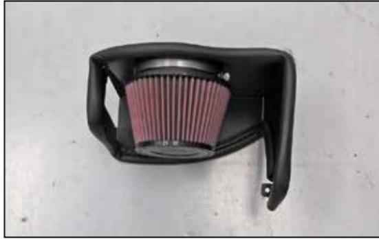
12. Install one of the provided air filters onto the driver side filter adapter as shown and secure with the provided hose clamp.
