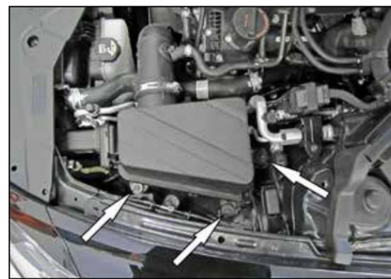
5. Remove the three bolts that secure the driver side air filter housing to the inner fender, loosen the hose clamp that secures the intake tube to the air filter housing and disconnect the tube. Remove the driver side air filter housing from the vehicle.
