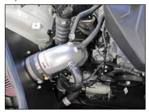
15. Connect the vent lines to the  $K\&N^{\otimes}$  intake tube as shown.
