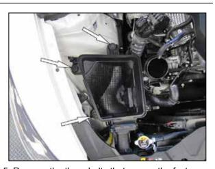
5. Remove the three bolts that secure the factory lower air filter housing to the inner fender and then remove the housing from the vehicle.
