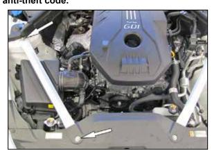
2. Remove the two bolts that secure the passenger side chassis brace and then remove the brace from the vehicle.
