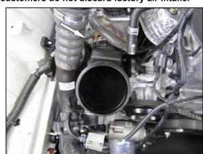
6. Loosen the hose clamp that secures the turbo inlet tube to the turbo and then remove the tube from the vehicle.
