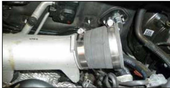
14. Install the provided coupler (08096) onto the turbo inlet and secure with the provided hose clamp.
