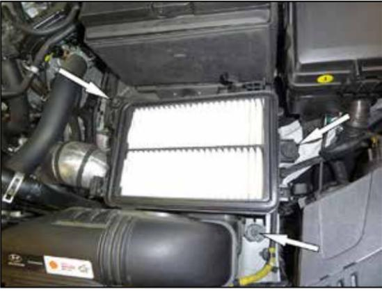
7. Remove the three bolts that secure the lower air filter housing and then remove the housing from the vehicle.
