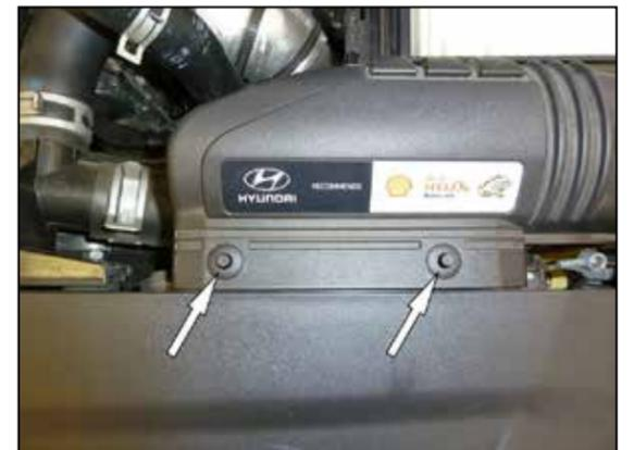
6. Push in the center of the fresh air intake duct retaining pins and then remove the pins from the vehicle.
