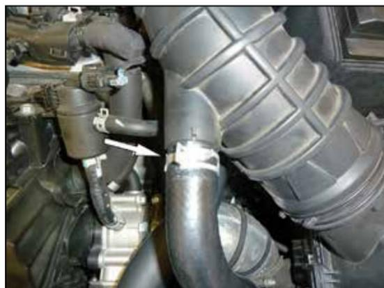
4. Release the spring clamp that secures the BOV hose to the intake tube and then disconnect BOV hose from the intake tube.
