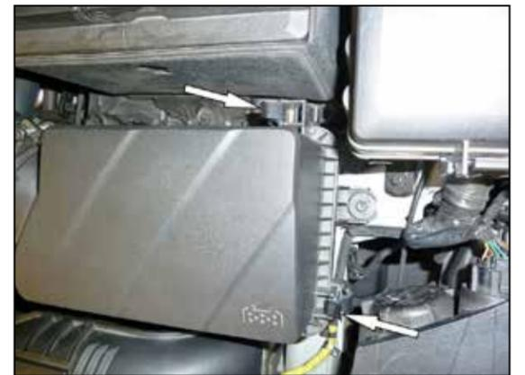
5. Release the two spring clips that secure the upper air filter housing and then remove the upper air filter housing and intake tube from the vehicle.
