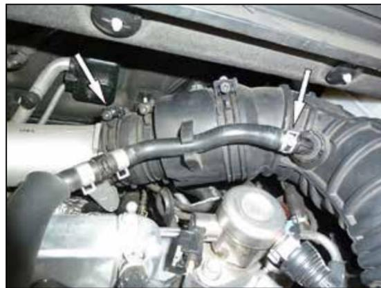
3. Release the spring clamp that secures the PCV vent line and then disconnect PCV line from the intake tube and unhook it from the clip. Loosen the hose clamp that secures the intake to the throttle body.
