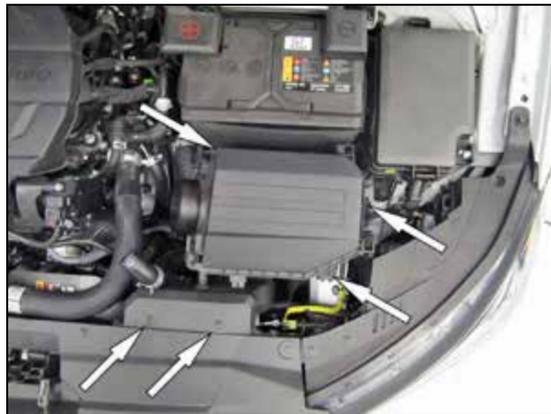
4. Remove the two plastic retaining clips that secure the fresh air intake duct. Remove the three bolts that secure the air filter housing and then remove the assembly from the vehicle.
