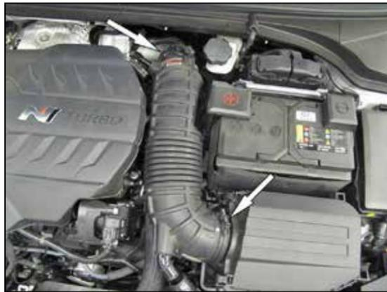
3. Loosen the two hose clamps that secure the factory intake tube and then remove the intake tube from the vehicle.
