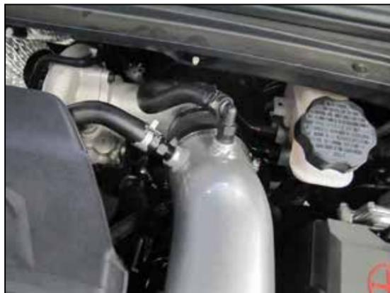
14. Connect the factory vent lines to the fittings installed into the K&N® intake tube and secure with the factory spring clamps.
