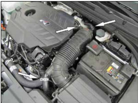
2. Release the spring clamps that secure the breather hoses and BOV hose and then disconnect them from the factory intake tube.
