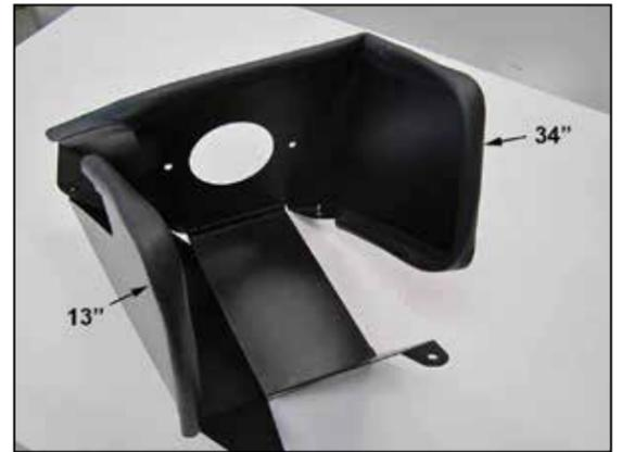
5. Cut the provided edge trim into sections of 13" and 34", install the edge trim onto the heat shield as shown.
