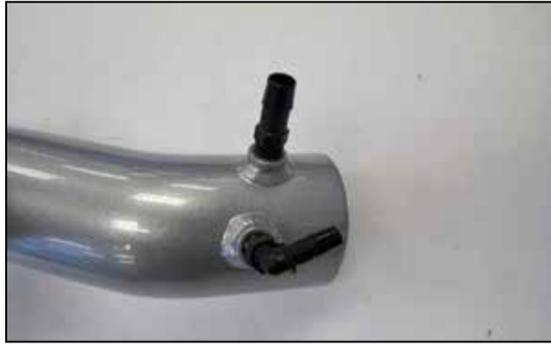
12. Install the provided vent fittings into the K&N® intake tube as shown.
