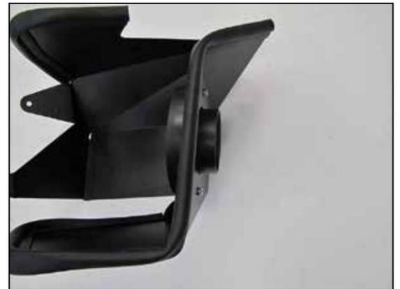
6. Install the filter adapter into the heat shield as shown and secure with the provided hardware.
