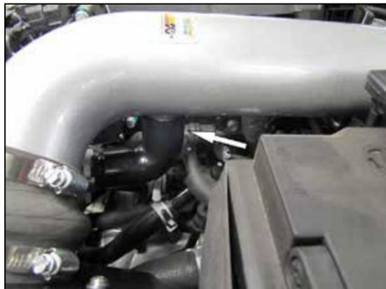
15. Connect the BOV elbow to the K&N® intake tube as shown.
