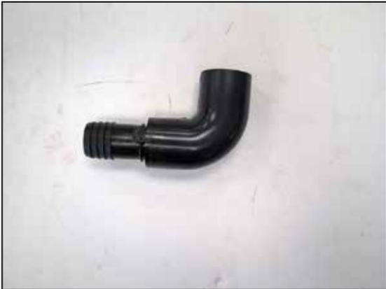
10. Install the provided union fitting into the elbow as shown.
