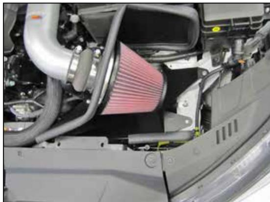
16. Install the K&N® air filter and secure with the provided hose clamp.
