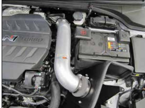
13. Install the K&N® intake tube into the coupler at the turbo and then into the coupler at the filter adapter, align the tube for best fit and then secure with the provided hose clamp.
