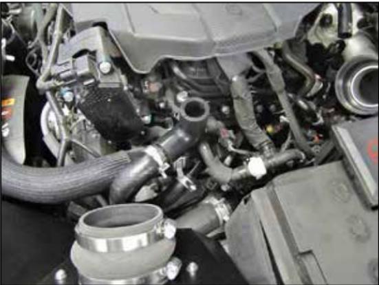
11. Install the elbow assembly into the factory BOV hose as shown.
