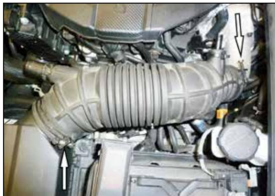
3. Loosen the hose clamps that secure the factory intake tube and then remove the tube from the vehicle.
