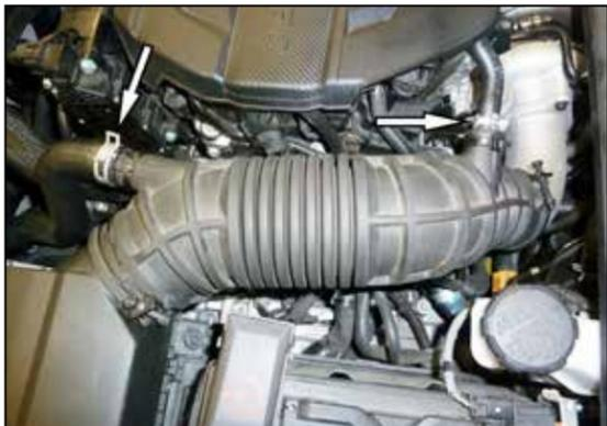
2. Release the spring clamps and then disconnect the CCV hose and BOV hose from the intake tube.
