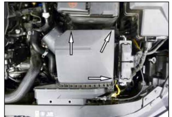
5. Remove the three bolts that secure the air filter housing and then remove the housing from the vehicle.
