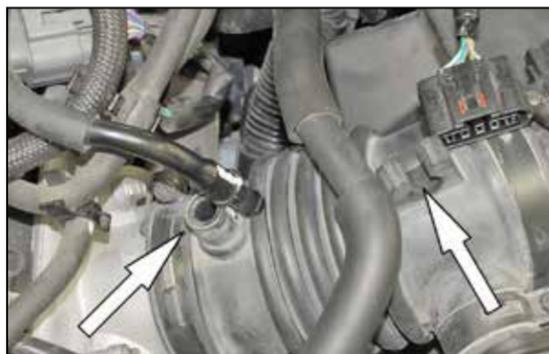
3. Disconnect the crank case vent hose and the EVAP vent hose from the factory intake tube.
