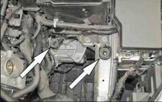
8. Remove the two air box mounting grommets shown. Install the provided rubber mounted stud onto inward air box mounting location.
