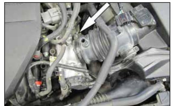
6. Loosen the hose clamp securing the factory intake tube to the throttle body.
