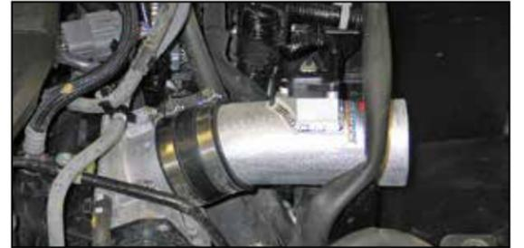
19. Install the K&N intake tube assembly into the hose at the throttle body and align with the mounting bracket. Secure the tube with the hardware and hose clamp provided.
