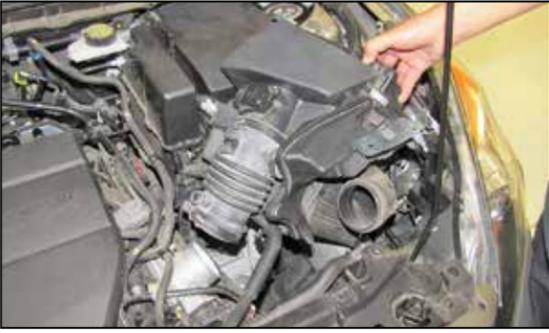
7. Lift up the air box to disconnect it from the mounting grommets, then disconnect the fresh air duct and remove the air box from the vehicle.
