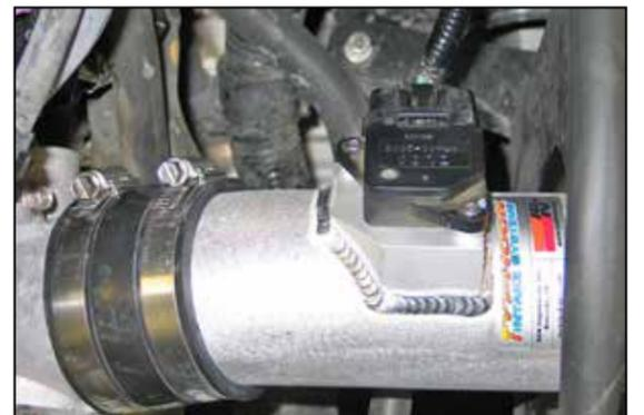
23. Reconnect the mass air sensor electrical connection.
