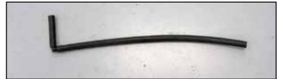
20. Install the two provided crank case vent hoses onto the 90° fitting as shown.
