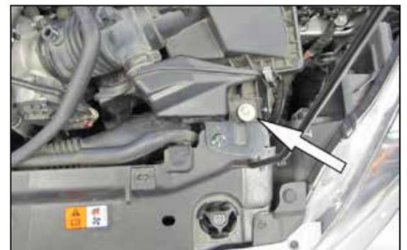
5. Remove the bolt shown securing the air box mounting bracket to the core support.
