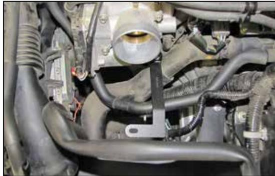
14. Install the tube mounting bracket onto the throttle body and secure with the factory bolt from the previous step.
