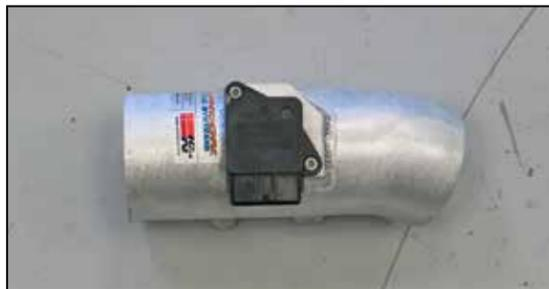
16. Install the mass air sensor into the K&N intake tube and secure with the provided hardware.
