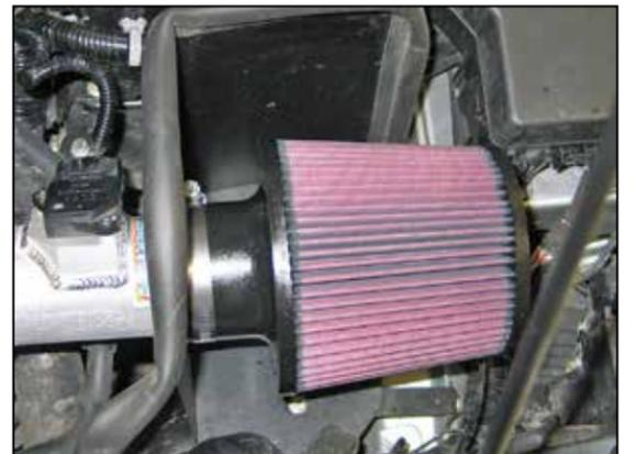
22. Install the K&N air filter onto the K&N intake tube and secure with the provided hose clamp.
