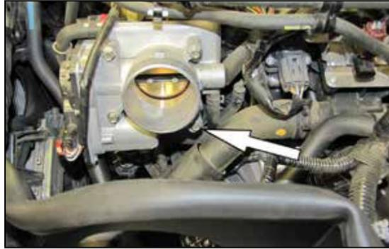
13. Remove the lower rear throttle body mounting bolt shown.
