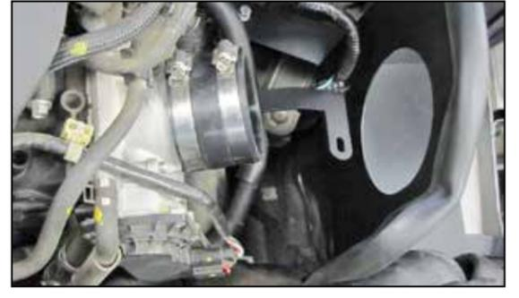
18. Install the provided coupling hose (08756) onto the throttle body and secure with the provided hose clamp.
