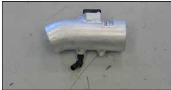
17. Install the 90° vent fitting into the K&N intake tube as shown.
