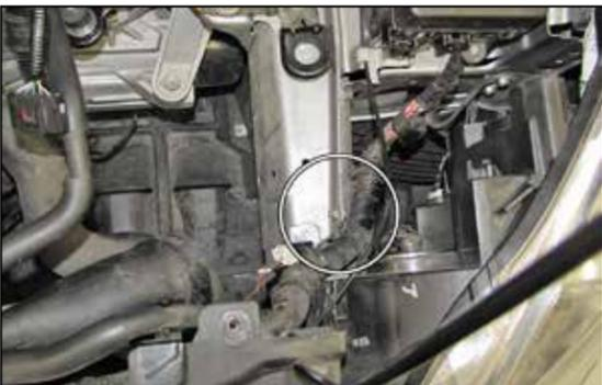
11. Remove the factory body bolt shown from the inner fender.
