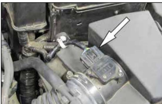
2. Disconnect the mass air sensor electrical connection and then unhook the wiring harness from the air box.
