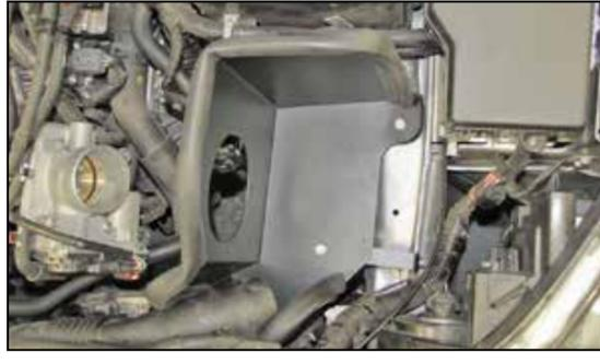
12. Install the heat shield assembly and secure with the provided hardware.
