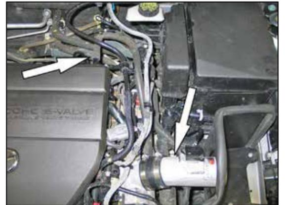
21. Connect the long end of the crank case vent hose to the fitting installed into the K&N intake tube and then attach the open end to the valve cover port.
