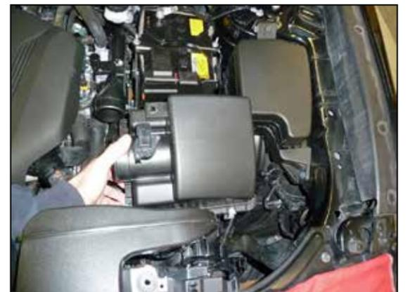
5. Pull straight up on the air filter housing assembly and remove it from the vehicle.
