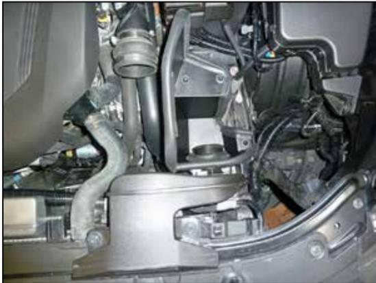
14. Install the heat shield assembly into the vehicle so the mounting grommets secure over the factory mounting studs. Secure the fresh air scoop with the factory bolts.
