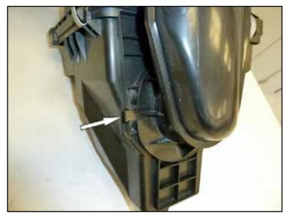
6. Lift the locking tab and then rotate the fresh air scoop counter clockwise to remove it from the air filter housing.
