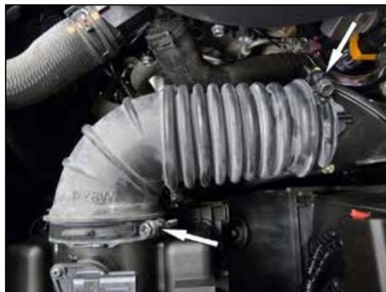
3. Loosen the clamps that secure the factory intake hose and then remove the factory hose from the vehicle.
