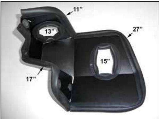
9. Install the cut edge trim onto the heat shield as shown.
