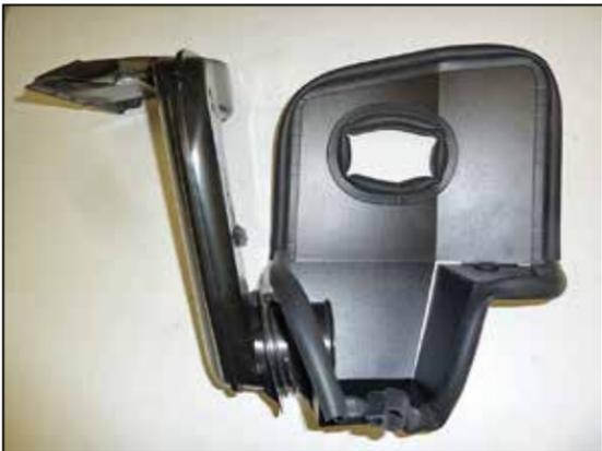
10. Install the factory fresh air intake scoop into the K&N® heat shield as shown.
