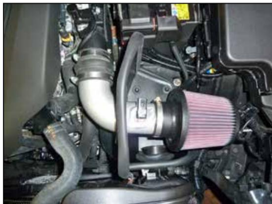
15. Install the K&N® intake tube through the heat shield, adjust for best fit and secure with the provided hose clamp.
