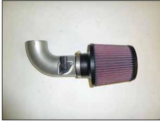
12. Install the air filter onto the K&N® intake tube and secure with the provided hose clamp.
