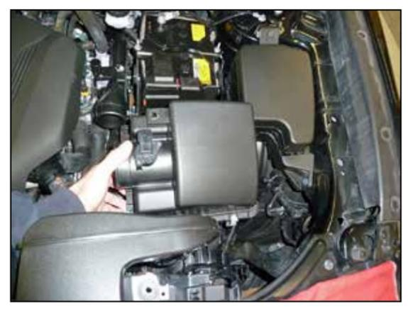
5. Pull straight up on the air filter housing assembly and remove it from the vehicle.
