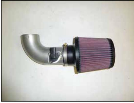
12. Install the air filter onto the K&N® intake tube and secure with the provided hose clamp.
