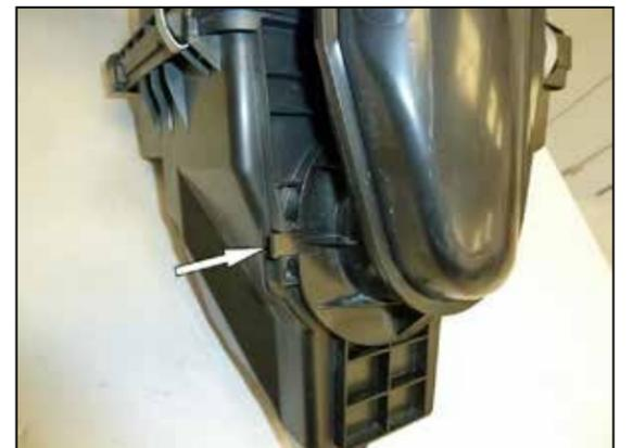
6. Lift the locking tab and then rotate the fresh air scoop counter clockwise to remove it from the air filter housing.
