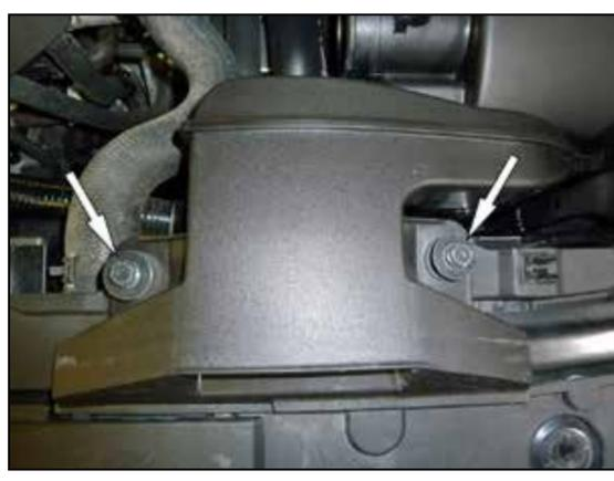
4. Remove the two bolts that secure the fresh air intake scoop to the core support.
