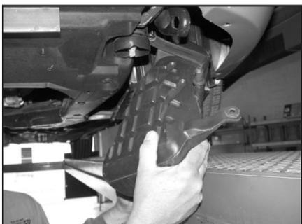
17. From underneath the vehicle, loosen and remove the two bolts that secure the intake resonator, then remove the resonator as shown.
