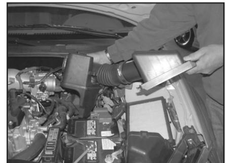
9. Remove the upper air cleaner assembly as shown.
