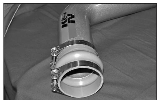
29. Install the stepped hump hose onto the cold air tube and secure it with the provided hose clamps as shown.
