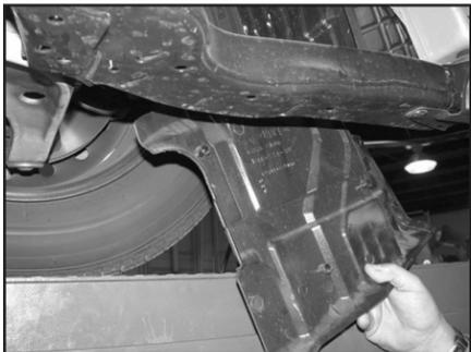
13. Remove the inner fender valance as shown.
