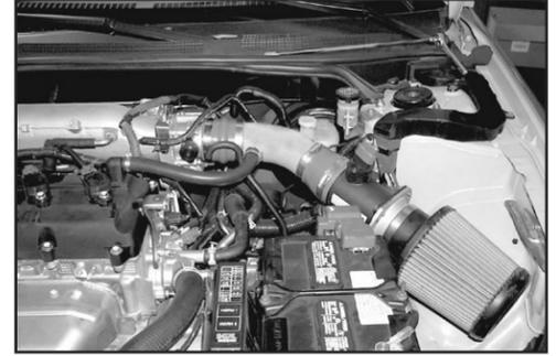
42. This intake kit has been designed to be used in two different configurations. In the case of inclement weather, the cold air tube can be removed and the air filter can be clamped onto the intake tube located in the engine compartment to avoid the possibility of ingesting water into the engine.
