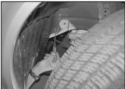
15. Remove the push clip from the inner wheel house valance as shown.
