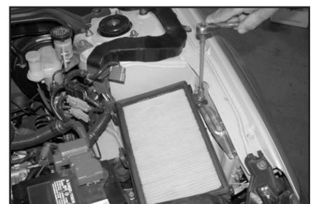
10. Loosen and remove the bolt that secures the lower air cleaner assembly as shown.
