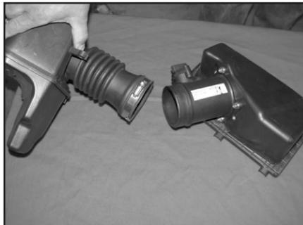
18. Loosen the hose clamp, then, remove the rubber bellows from the mass air sensor as shown.
