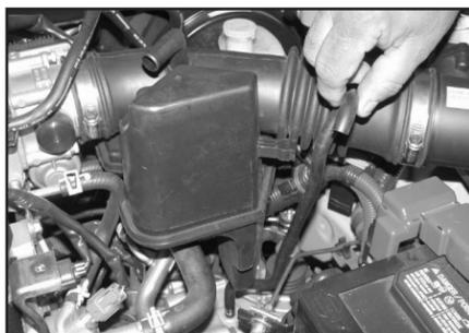
5. Remove the transmission vent hose from the resonator as shown.
