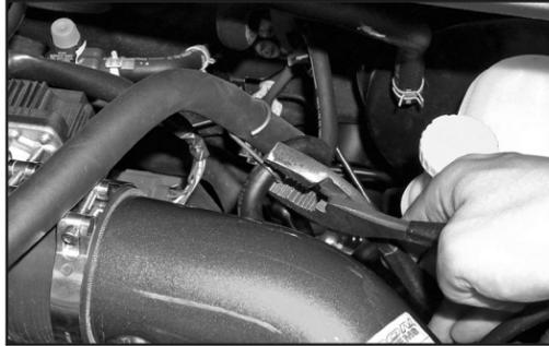
37. On 2005 models, open the supplied cable support clip and route over the fuel line hose. Clamp cable support clip to tighten if necessary.
