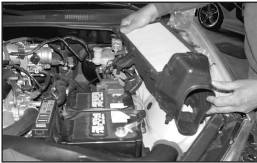
11. Pull firmly upwards to release and remove the lower air cleaner assembly as shown.
