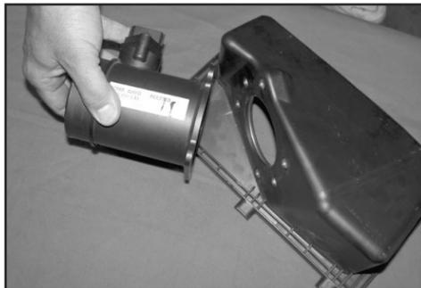
19. Loosen and remove the four bolts that secure the mass air sensor, then, remove the mass air sensor as shown.
