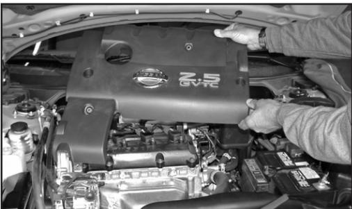
2. Remove the four bolts that retain the engine cover, then remove the engine cover.
