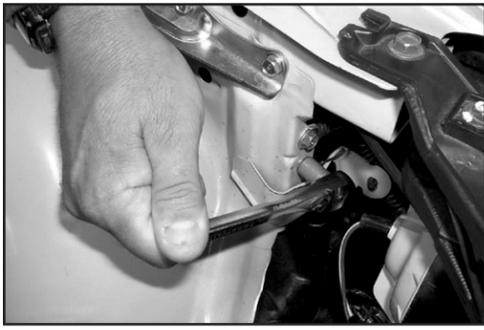
30. Loosen and remove the lower bolt that secures the ground wire to the inner fender as shown.
