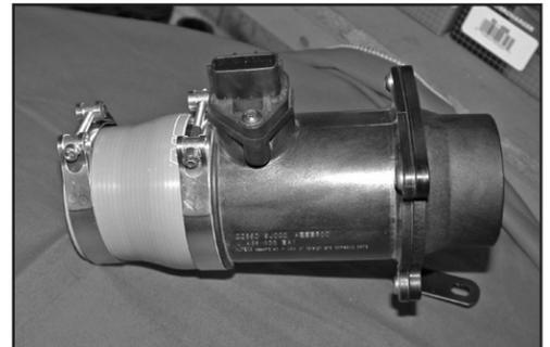
24. Install the silicone hose and hose clamps onto the mass air sensor as shown.
