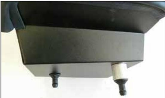
10. Install the heat shield mounting studs as shown using the provided hardware and spacer.
