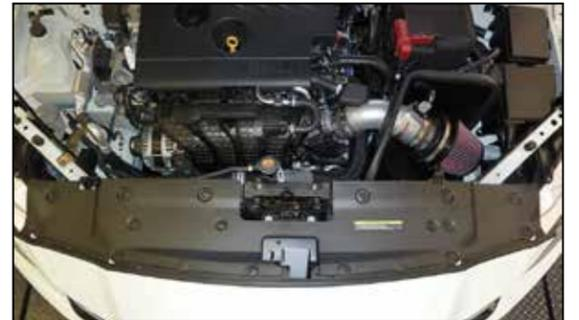
20. Reinstall the valence and secure with the factory retaining clips.
