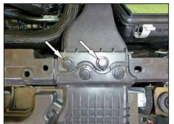
6. Remove the two plastic clips that retain the fresh air intake duct and then remove the duct from the vehicle.
