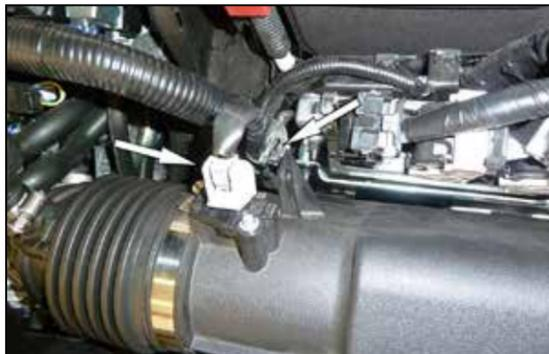
3. Disconnect the mass air sensor electrical connection and then unhook the harness from the air filter housing and engine.
