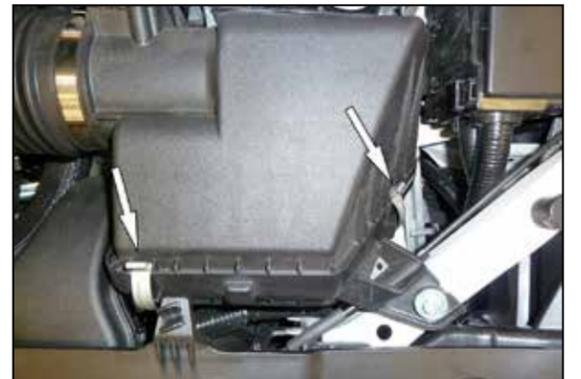
5. Release the two upper air filter housing retaining clips and then remove the upper air filter housing and intake boot from the vehicle.
