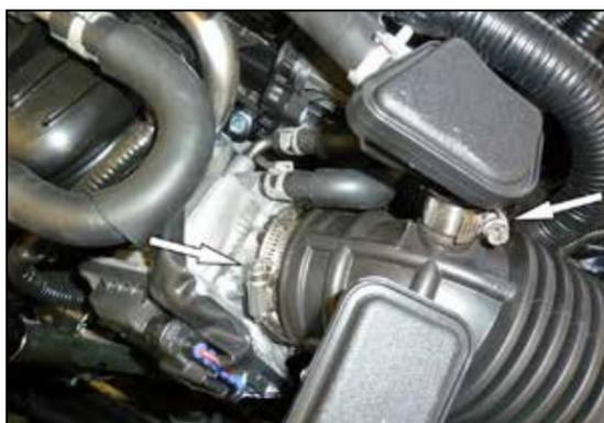
4. Loosen the clamp that secures the PCV chamber to the intake boot and then separate the chamber from the intake boot. Loosen the hose clamp that secures the intake boot to the throttle body.
