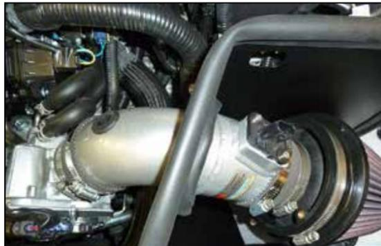
17. Install the intake tube through the heat shield and into the coupler at the throttle body, adjust the tube for best fit and then secure with the provided hose clamp.
