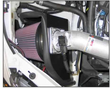
18. Reconnect the mass air sensor electrical connection as shown.
