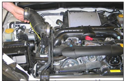
4. Loosen the two hose clamps which secure the factory intake tube and then remove the intake tube from the vehicle.
