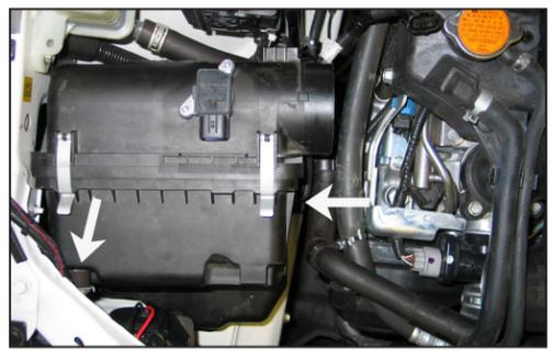
5. Loosen and remove the two bolts which secure the airbox to the inner fender.
