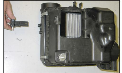
8. Remove the two screws which secure the mass air sensor and then remove the mass air sensor from the airbox as shown.
