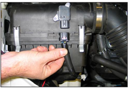
3. Disconnect the mass air sensor electrical connection and then unhook the wiring harness from the airbox.
