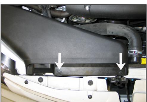
2. Remove the two fasteners which retain the fresh air inlet scoop and then remove the fresh air inlet scoop from the vehicle as shown.
