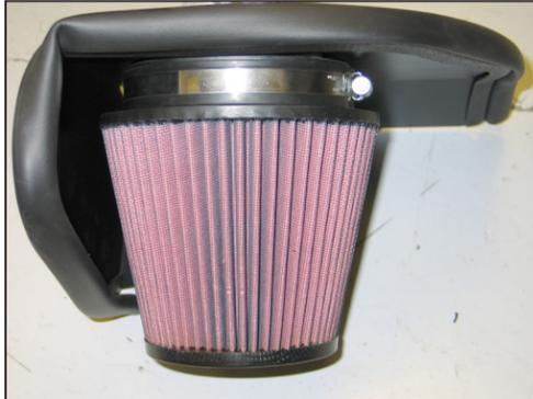
15. Install the K&N® air filter onto intake assembly and secure with the provided hose clamp.
