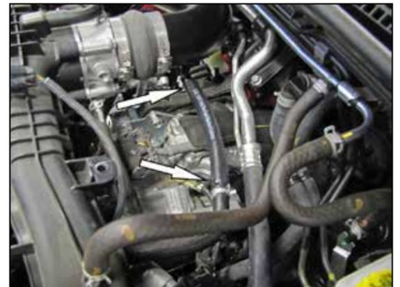
21. Install the K&N® crank case vent hose onto the fitting installed into the intake tube and then connect the union to the factory crank case vent hose.
