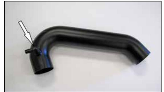
18. Install the provided 90° vent fitting into the K&N® intake tube as shown.
