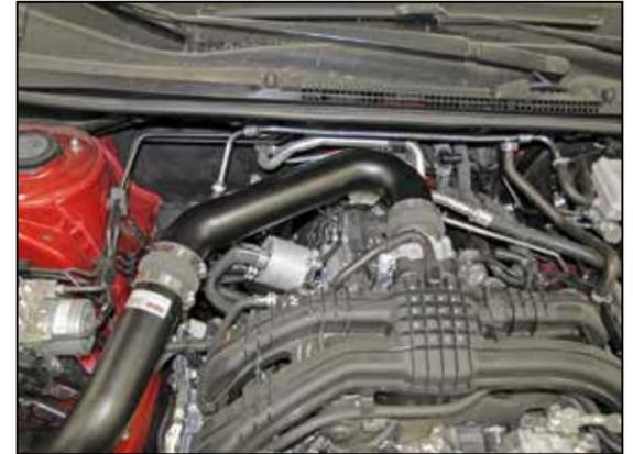
19. Install the K&N® intake tube into the hump couplers, adjust both tubes for best fit and then secure the hose clamps and the tube mount to the heat shield.
