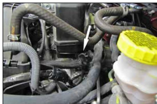
3. Disconnect the crank case vent line from the intake plenum.
