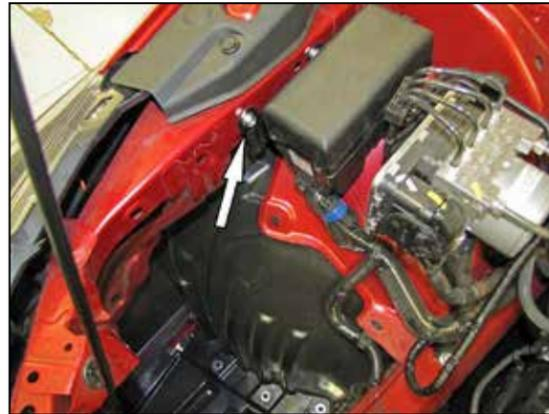
15. Remove the bolt that secures the electrical junction block to the inner fender.
