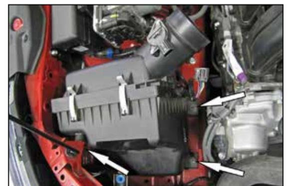
6. Remove the one nut and two bolts that secure the air filter housing and then remove the housing from the vehicle.
