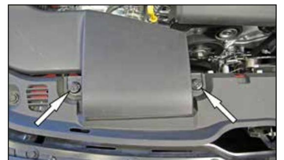
5. Remove the two retaining clips and then remove the fresh air duct from the vehicle.
