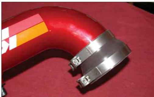
12. Install the silicone hose and hose clamps onto the intake tube as shown.
