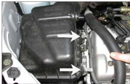
4. Unclip the upper air cleaner assembly as shown.
