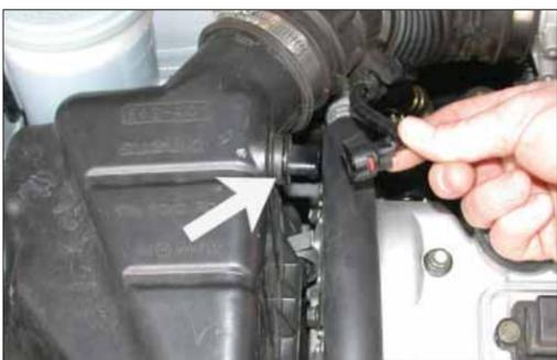
2. Disconnect the air temperature sensor electrical connection as shown.
