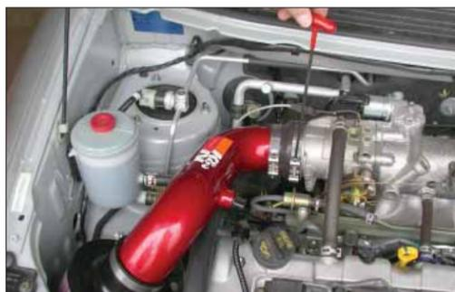
16. Tighten the hose clamp on the throttle body as shown.
