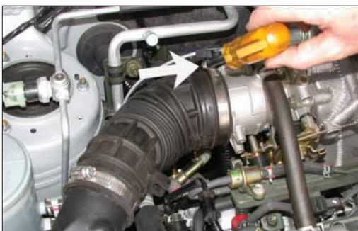
3. Loosen the hose clamp at the throttle body as shown.
