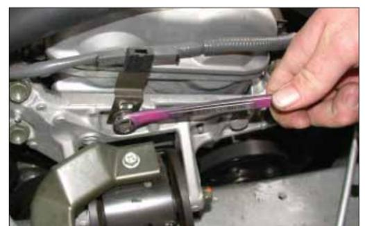
9. Remove the bolt that secures the wire harness bracket to the engine mount bracket as shown.
