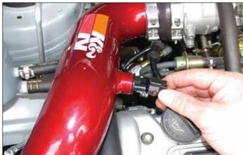
17. Reconnect the air temperature sensor electrical connection as shown.
