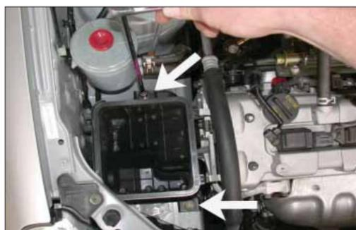
6. Remove the two bolts that secure the lower air cleaner assembly.
