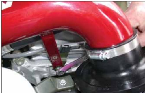
15. Line up the bracket with the threaded hole from step 9 and secure with the stock bolt from step 9.
