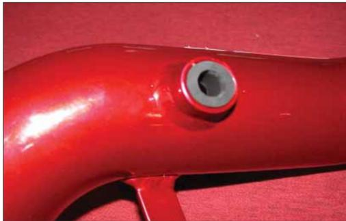
10. Install the silicone hose into the vent on the Typhoon intake tube as shown.
