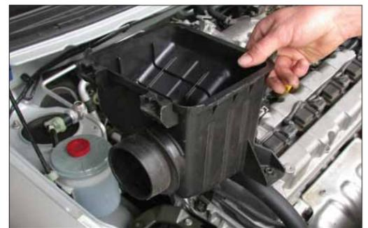
7. Remove the lower air cleaner assembly as shown.
