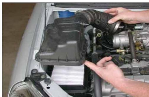
5. Pull the stock intake hose off the throttle body and remove the upper air cleaner assembly as shown.
