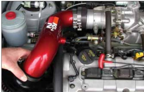
14. Install the intake tube assembly onto the throttle body as shown.
