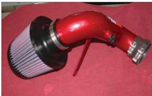
13. Install the air filter onto the intake tube as shown.
