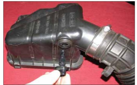
8. Remove the air temperature sensor from the upper air cleaner assembly as shown.
