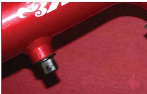
11. Install the air temperature sensor into the silicone hose on the intake tube as shown.
