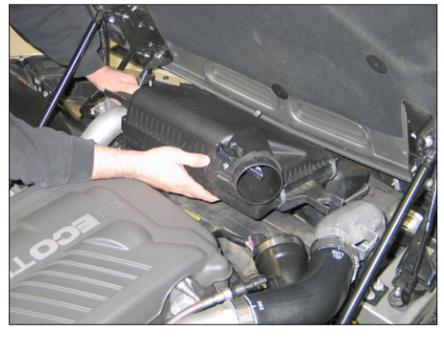
8. Pop the air box assembly up to release it from the mounting grommets, slide the air box assembly to the right side of the vehicle, pull the left side intercooler tube to the left and then pull up the air box flange around the intercooler tube. Once the air box is clear of the intercooler tubes, tip the back side up towards the hood so the front will clear the hood and then remove the complete air box assembly.
