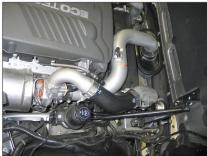
19. Install the K&N® intake tube into the silicone hose at the turbo inlet and align with the mounting bracket installed in step #14, slide the filter onto the end of the intake tube. Secure the intake tube with the provided hose clamp and hardware. Secure the filter with the provided hose clamp.
