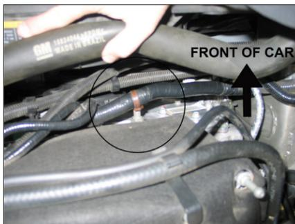
13. Unhook the engine wiring harness from the stud on the front of the engine.
