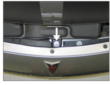
5. Remove the bolt which secures the front of the factory air box to the frame.
