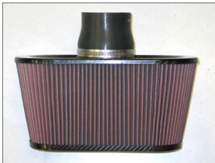
17. Install the provided silicone hose (084055) onto the K&N® air filter and secure with the provided hose clamp.
