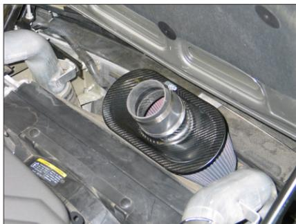
18. Set the K&N® filter assembly into position on the radiator shroud as shown.
