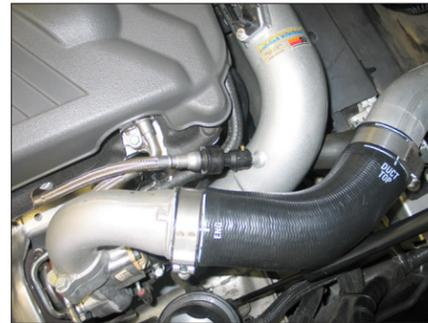
20. Connect the crank case vent fitting to the fitting on the K&N® intake tube.
