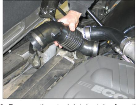
9. Remove the stock intake tube from the vehicle. **NOTE: K&N Engineering, Inc., recommends that customers do not discard factory air intake.**
