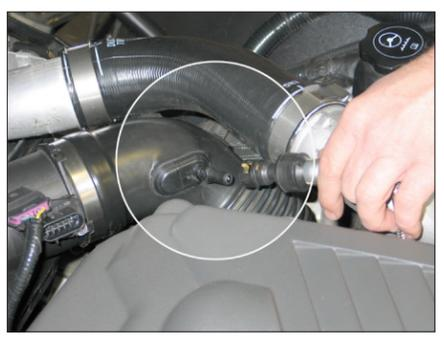
3. Release the crank case vent line retaining clip and then disconnect the crank case vent line.
