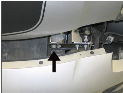
10. Reinstall the bolt which secures the left side intercooler tube to the front mounting bracket.
