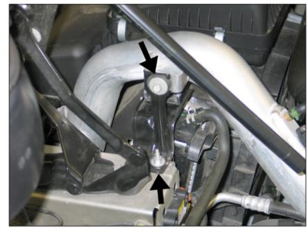
6. Remove the two bolts which secure the left side intercooler tube mounting bracket and then remove the bracket.
