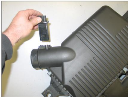
15. Remove the mounting screws and then remove the mass air sensor from the stock air box.
