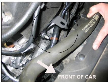
14. Install the tube mounting bracket (083122) onto the stud on the front of the engine and secure with the hardware. Re-secure the wiring harness to the stud after the bracket has been installed.
