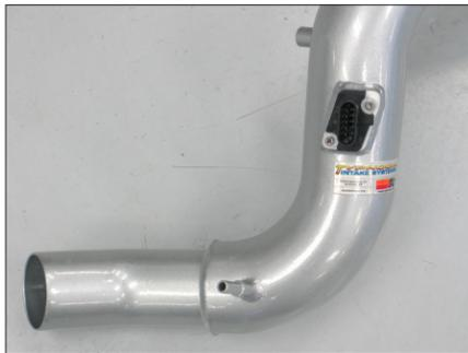
16. Install the mass air sensor into the K&N® intake tube and secure it with the provided hardware.
