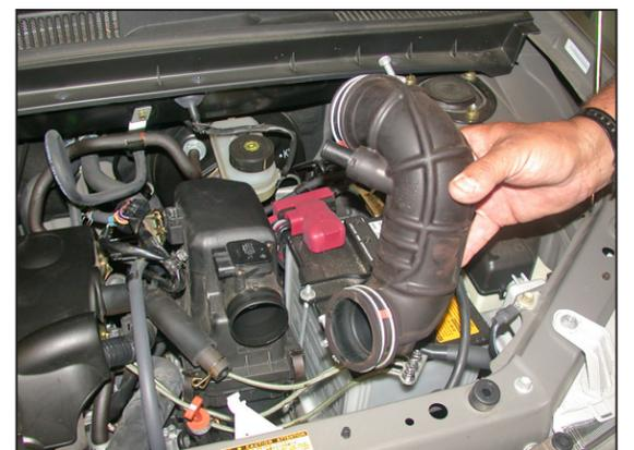
5. Loosen the hose clamps at the throttle body and at the air cleaner assembly, then, remove the stock intake tube as shown.
