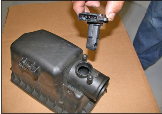
21. Remove the mass air sensor from the upper air cleaner assembly as shown.
