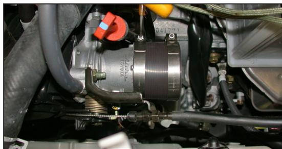
16. Install the silicone hose and hose clamps onto the throttle body and tighten as shown.
