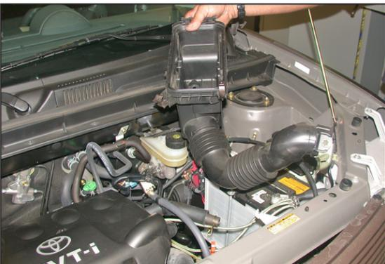
9. Pull upwards to remove the lower air cleaner assembly as shown.
