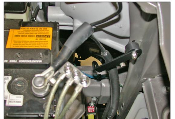
20. Secure the short "L" bracket to the rubber mounted stud from the previous step using the provided hardware but do not tighten at this time.
