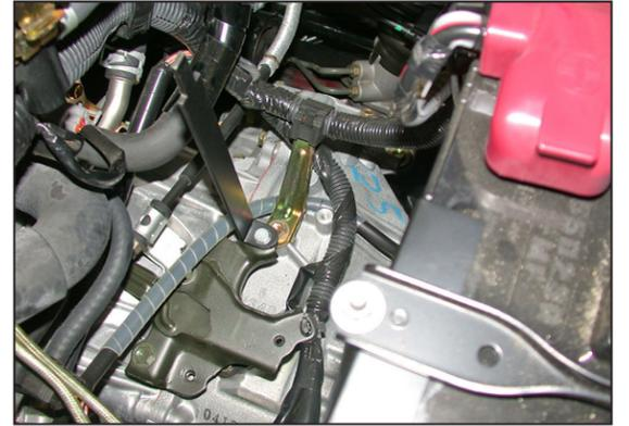
17. Using the provided hardware secure the provided large "L" bracket to the original air cleaner mounting bracket as shown.
