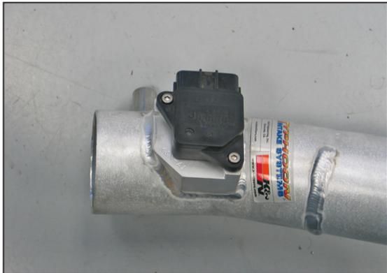
22. Install the stock mass air sensor into the K&N® Typhoon® cold air tube and secure with the provided hardware as shown.
