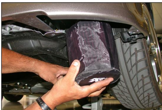
31. From underneath the vehicle pull the inner fender valance down, then, slide the Air filter onto the cold air tube and secure with the provided hose clamp.
