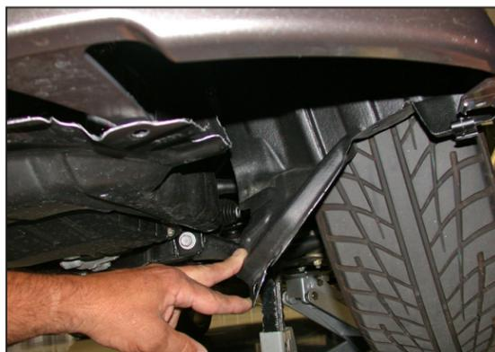
15. Remove the plastic rivet from the inner fender valance as shown.
