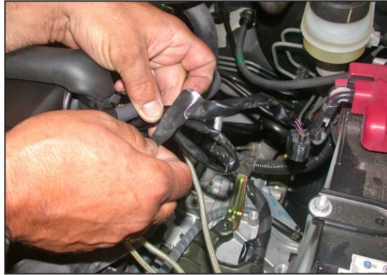
11. Remove the tape that binds the three wire harnesses together.
