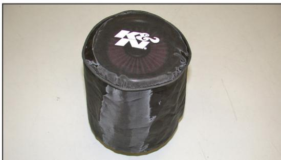
30. Install the K&N® Drycharger onto the K&N® Air filter as shown.
