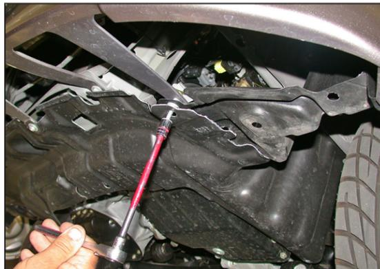
14. Remove the two screws that secure the inner fender valance.
