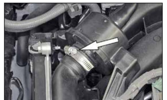
5. Loosen the hose clamp and disconnect the engine sound tube from the engine sound drum.
