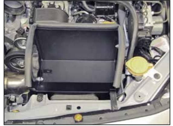
17. Set the heat shield into position on the core support and secure with the factory air box mounting bolts and to the previously installed bracket with the hardware provided.
