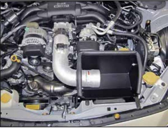
22. Rotate the tube down and install it into the silicone hose on the throttle body and install the mounting stud into the bracket. Secure the tube with the provided hose clamps and hardware and tighten the mounting bracket at this time.
