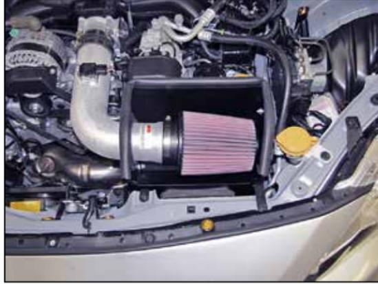
25. Install the K&N® air filter onto the K&N® intake tube and secure with the provided hose clamp.
