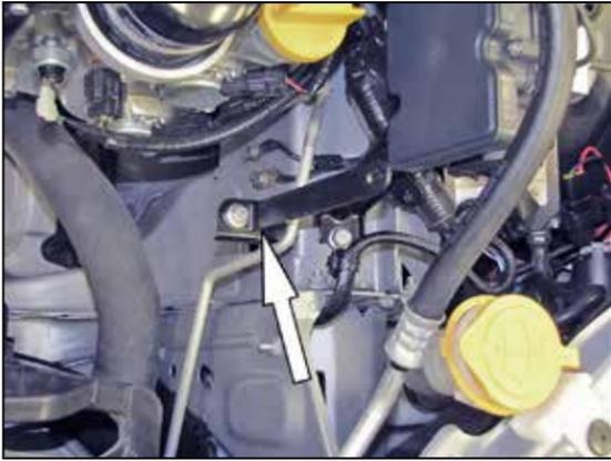
8. Install the provided heat shield mounting bracket (070026A) onto the lower air box mount using the factory bolt.
