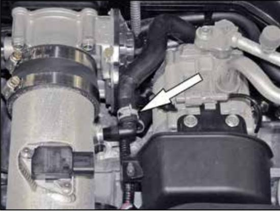
23. Connect the crank case vent to the fitting installed into the K&N® intake tube as shown.
