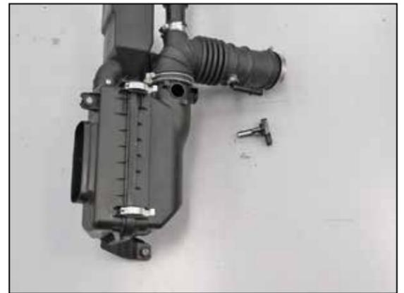
19. Remove the two screws securing the mass air sensor into the factory air box and then remove the mass air sensor from the air box.
