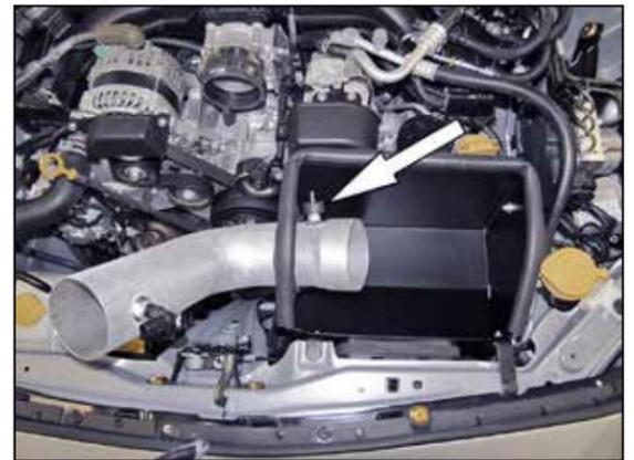
21. Install the tube through the heat shield and then install the provided rubber mounted stud onto the tube as shown.
