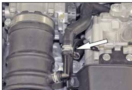
3. Release the spring clamp and then disconnect the crank case vent hose from the fitting.
