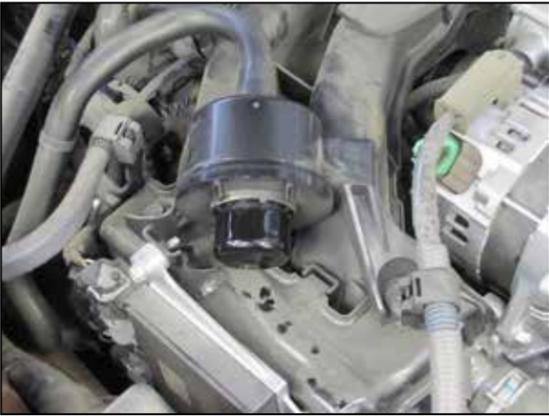
23a. Install the provided capplug onto the engine sound drum as shown.
