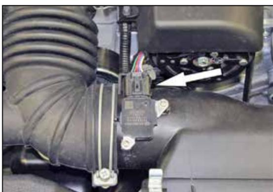
2. Disconnect the mass air sensor electrical connection and unhook the wiring harness from the air box.
