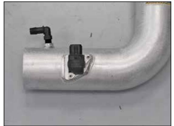
20. Install the mass air sensor into the K&N® intake tube and secure with the provided hardware.
