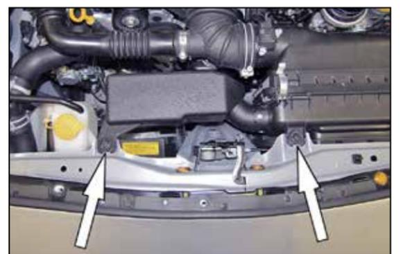
6. Remove the two bolts shown securing the resonator and air box to the core support.
