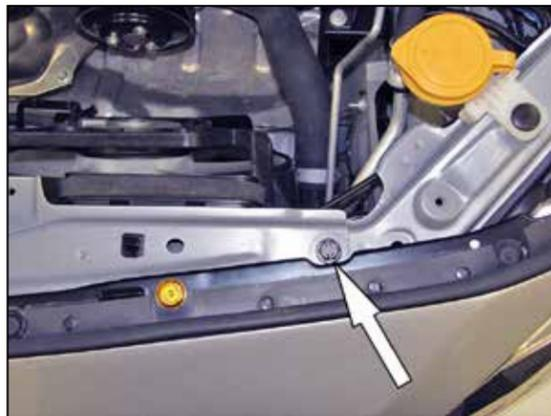
16. Remove the core support bolt shown.
