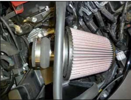
10. Install the provided hump coupler onto the filter adapter and secure with the provided hose clamp. Install the K&N® air filter onto the filter adapter and secure with the provided hose clamp.
