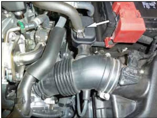
4. Release the spring clamp that secures the crank case vent hose to the plenum and then disconnect the hose from the plenum.
