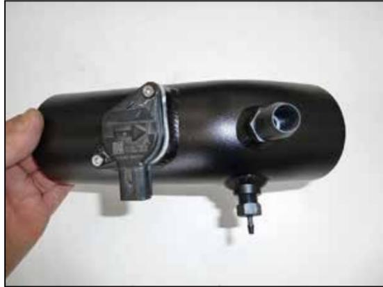
12. Remove the mass air sensor from the factory air filter housing and then install it into the K&N® intake tube and secure with the provided hardware. Install the two provided vent fittings into the K&N® intake tube as shown. **NOTE: NPT fitting has tapered threads and only designed to be installed until hand tight, then tighten one rotation or when the fitting becomes difficult to return.**
