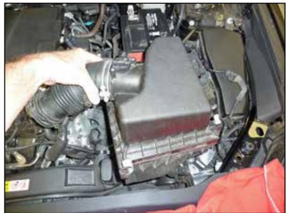
5. Lift the air filter housing up to dislodge it from the mounting grommets and remove the complete assembly from the vehicle. **NOTE: K&N Engineering, Inc., recommends that customers do not discard factory air intake.**
