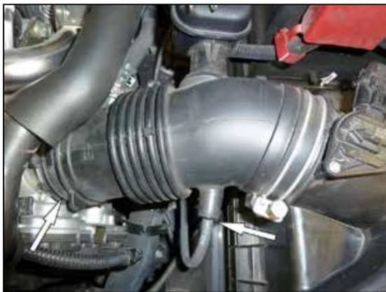
3. Release the spring clamp that secures the intake tube to the throttle body and then disconnect the hose from the throttle body. Disconnect the vacuum line from the intake tube.
