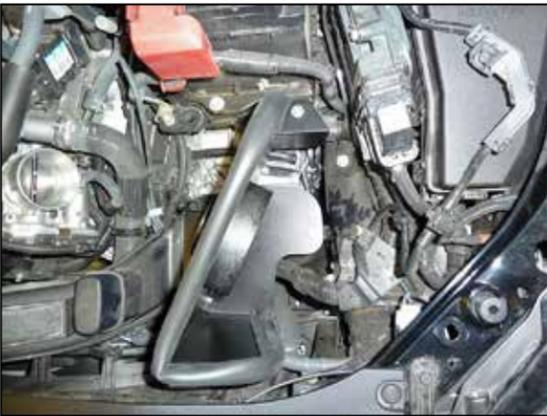
9. Install the heat shield assembly into the vehicle so that the mounting studs insert into the factory air filter housing mounting grommets.
