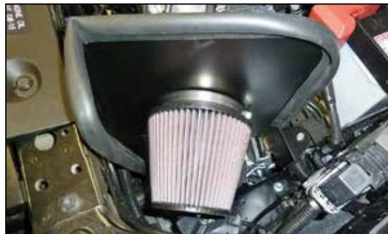
16. Install the K&N® air filter onto the filter adapter and secure with the provided hose clamp.
