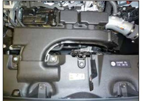
20. Reinstall the fresh air intake duct and secure with the factory hardware.
