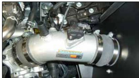
17. Install the K&N® intake tube assembly into the couplers and adjust for best fit and secure with the provided hose clamps.
