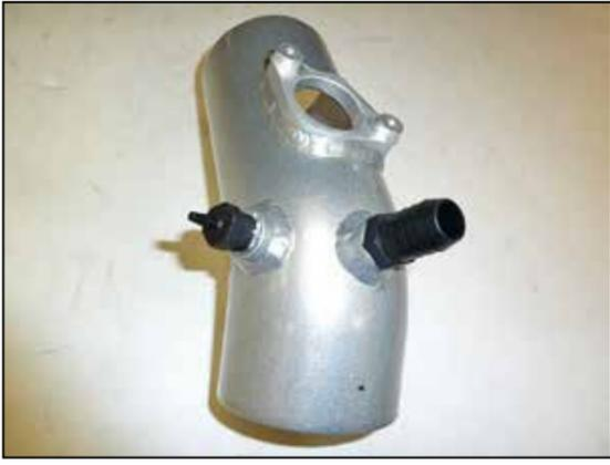
7. Install the provided vent fittings into the K&N® intake tube as shown.
