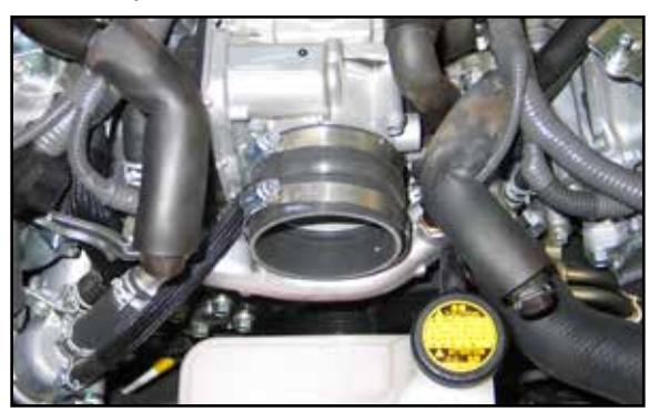
26. Install the provided silicone hose (084091) onto the throttle body and secure with the provided hose clamp.
