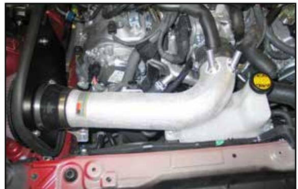
27. Install the K&N® intake tube into the silicone hose at the filter adapter, then into the silicone hose at the throttle body. Secure with the provided hose clamps.
