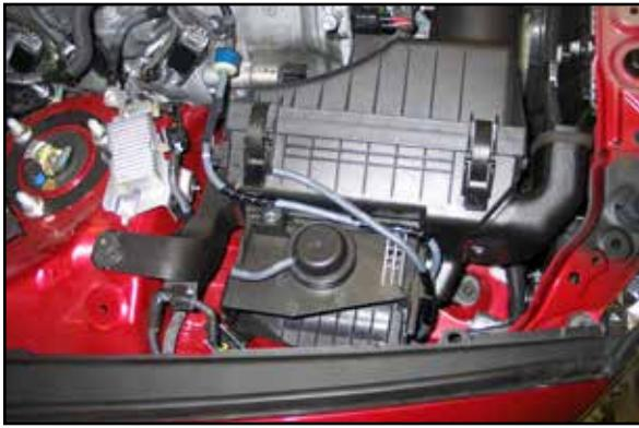
11. Remove the two bolts which secure the air box to the inner fender.
