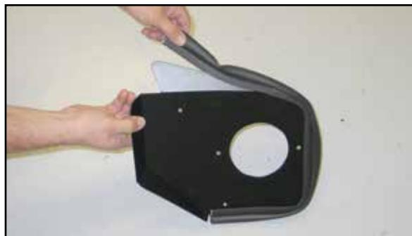
16. Install the long edge trim onto the heat shield as shown.
