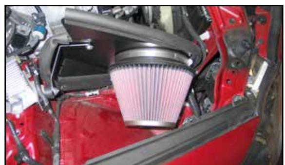
24. Install the K&N® air filter and secure with the provided hose clamp.
