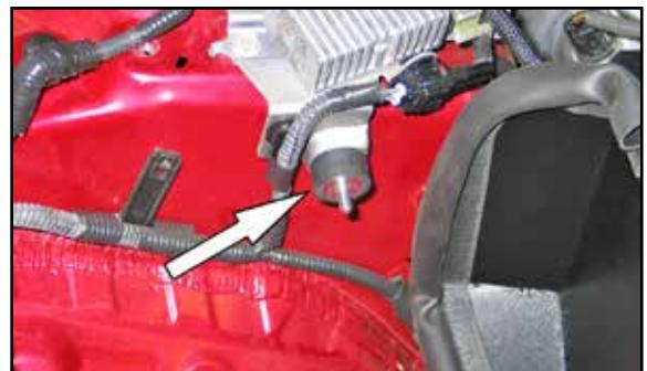
22. Install the provided rubber mounted stud into the module mounting bracket as shown.
