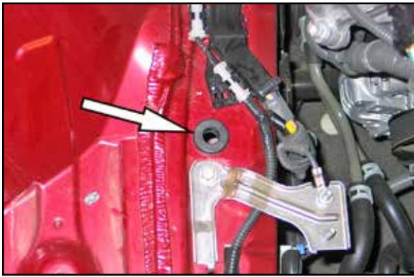
13. Remove the air box mounting grommet shown from the inner fender.
