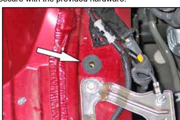
20. Install the inserted nut into the air box mounting grommet hole in the inner fender as shown.
