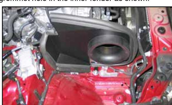
21. Install the heat shield assembly and secure the mounting bracket to the inserted nut installed in the previous step.
