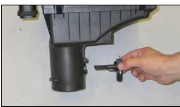
14. Remove the mass air sensor from the factory air box as shown.
