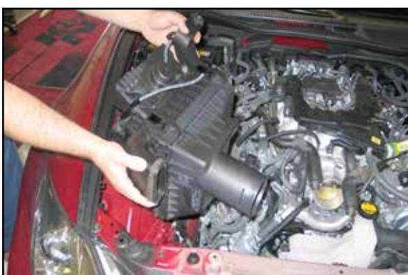
12. Lift up the air box to gain access to the remaining vacuum line connection and wiring harness clip. Disconnect the vacuum line and unhook the wiring harness from the air box. Remove the air box from the vehicle.
