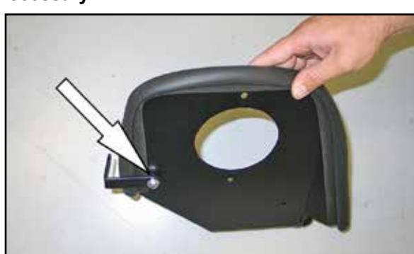
18. Install the heat shield mounting bracket (070111) onto the heat shield as shown.
