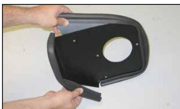
17. Install the short edge trim onto the heat shield as shown.
