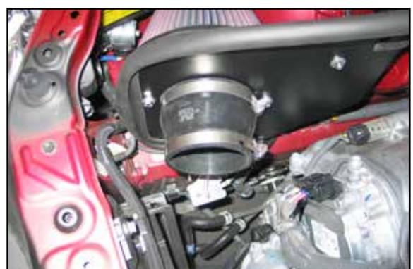
25. Install the silicone hose (08050) onto the filter adapter as shown and secure with the provided hose clamp.
