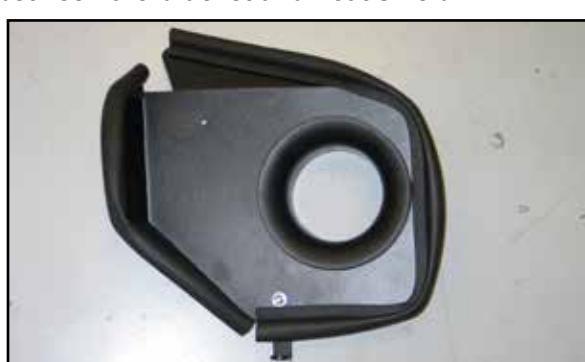
19. Install the filter adapter onto the heat shield and secure with the provided hardware.
