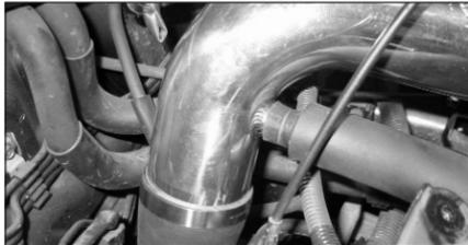
24. Mount the breather hose onto the new intake tube using the original hose clamp as shown.
