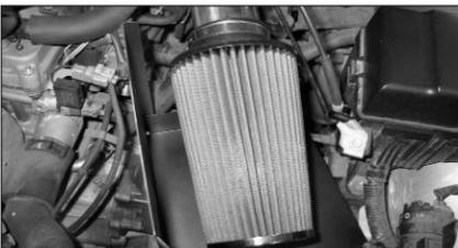
21. Mount the filter on the new intake tube using the #44 hose clamp supplied.
