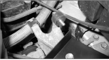
17. Mount the rubber vibration stud onto the gear box mounting bracket using the hardware supplied.
