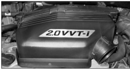
25. Refit the complete air box back onto the engine as shown.
