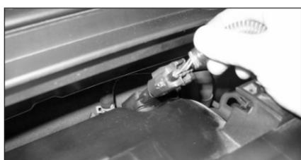
6. Disconnect the mass air sensor (MAS) electrical connection as shown.
