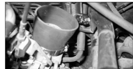
14. Install the silicone step hose and hose clamps supplied onto the throttle body as shown. Do not fully tighten yet!
