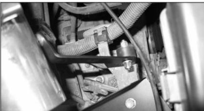
20. Mount the "L" bracket onto the rubber vibration stud using the hardware supplied. Do not fully tighten yet!
