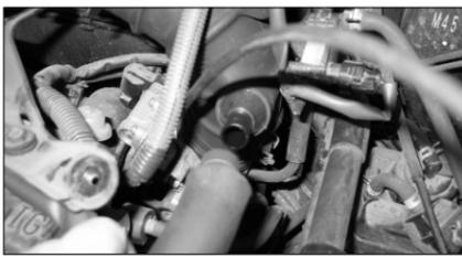
7. Unclip and remove the breather from the intake tube as shown.
