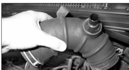
9. Remove the stock intake tube from the vehicle as shown.
