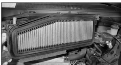
11. Remove the air box base from the vehicle as shown.
