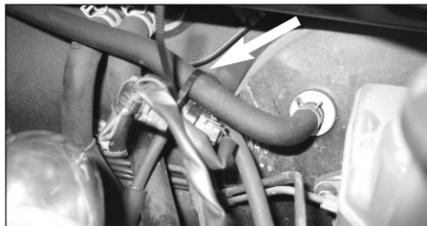
27. Fit the vacuum switch onto the big vacuum hose as shown, using a cable tie supplied.
