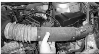
2. Unclip and remove the air inlet duct from the vehicle as shown.
