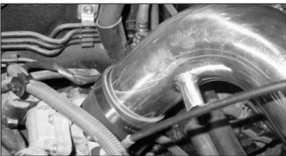
19. Mount the Typhoon tube into the silicone step hose, as shown. Do not fully tighten the hose clamp yet!
