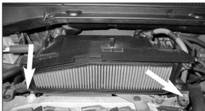
10. Loosen and remove the two bolts that secure the air box base to the engine as shown.
