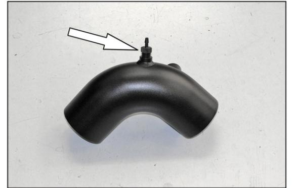
18. Install the provided vent fitting into the K&N® intake tube as shown.
