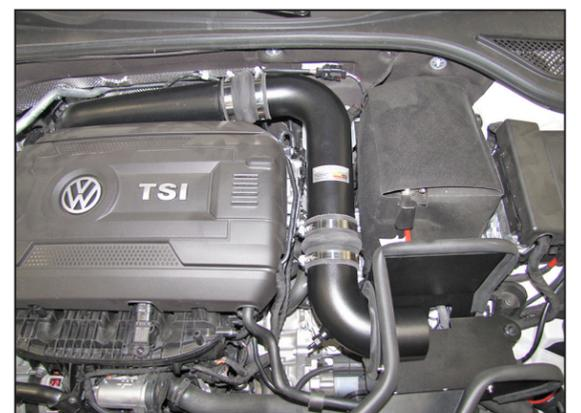
20. Install the primary intake tube onto the secondary tube and align with the mounting bracket installed onto the heat shield. Adjust the tubes for best fit and then secure with the provided hose clamps and hardware.
