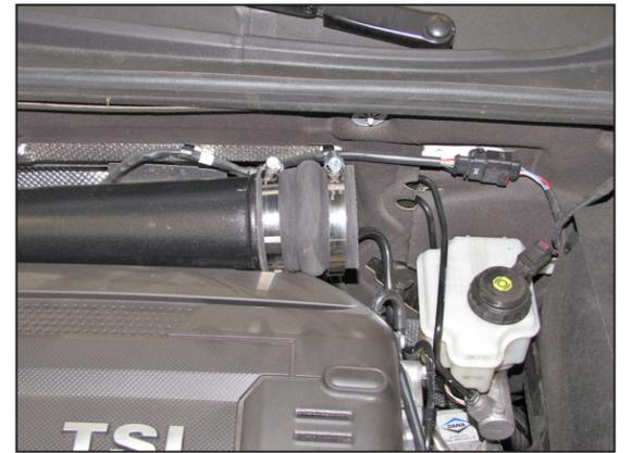
16. Install the provided coupling hump hose (08696) onto the turbo inlet and secure with the provided hose clamp.
