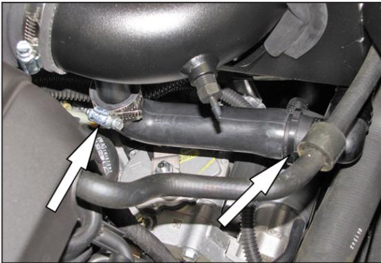
23. On vehicles that are equipped with air injection, Install the air injection hose assembly into the factory quick disconnect fitting and then install the open end onto the fitting installed on the intake tube. Secure the hose to the intake tube with the provided hose clamp. On vehicles that are not equipped with air injection, install the provided capplug onto the air injection port of the K&N® intake tube and secure with the provided hose clamp.
