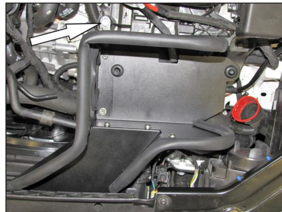
15. Install the heat shield assembly onto the mounting studs and secure the mounting bracket to the air filter housing with the provided hardware.
