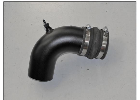
19. Install the remaining coupling hump hose (08696) onto primary K&N® intake tube and secure with the provided hose clamp.
