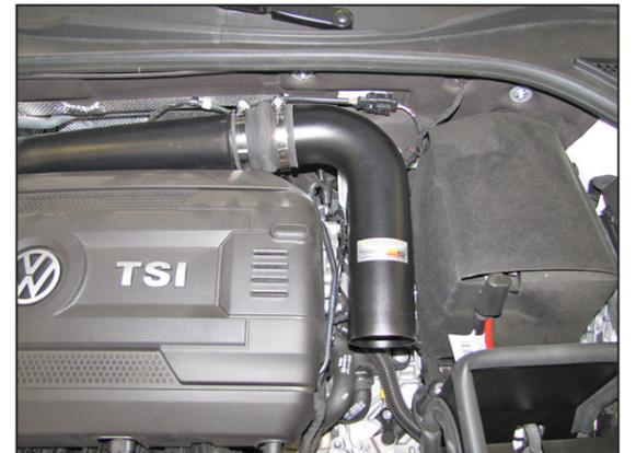
17. Install the secondary K&N® intake tube (27626) into the coupling hose at the turbo inlet and secure with the provided hose clamp.
