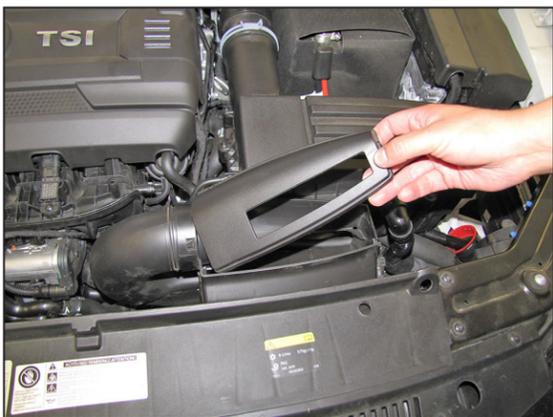
2. Release the fresh air intake scoop lid from the retaining tabs and then remove the lid from the fresh air intake scoop.
