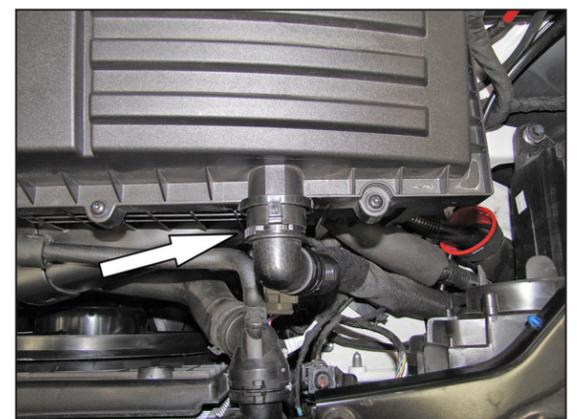
5. Disconnect the air injection hose from the upper air filter housing.
