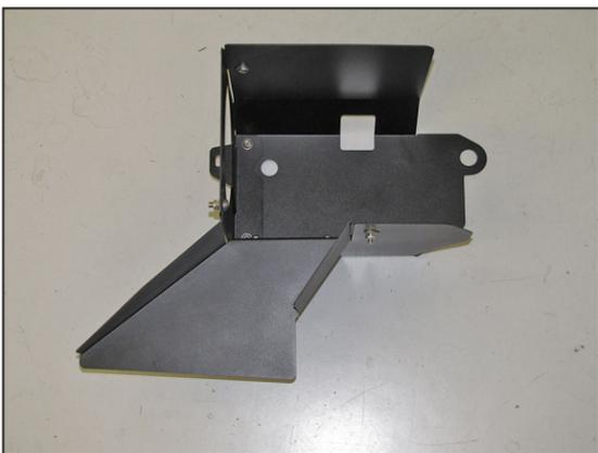
10. Install the provided fresh air intake scoop onto the heat shield and secure with the provided hardware.
