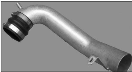
9. Fit the silicone hose on to the tube using the hose clamp supplied. NOTE: Before installing clean the inside of out with water and a towel!
