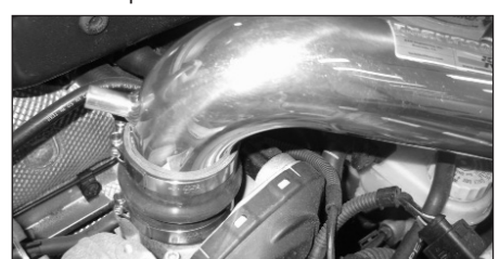
13. Fit the short ram intake tube on to the throttle body and secure the hose clamp.
