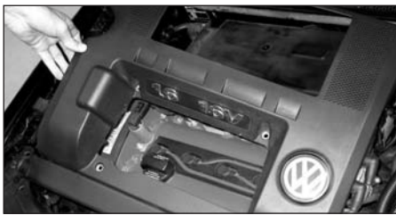
2. Remove the four Allen head bolts and carefully remove the plastic engine cover.
