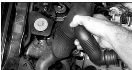
5. Unbolt and remove the pick up pipe.
