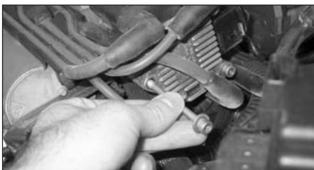
11. Remove the front bolt from the ignition amplifier.
