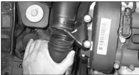
4. Unclip and remove the pick up pipe from the air box intake tube.
