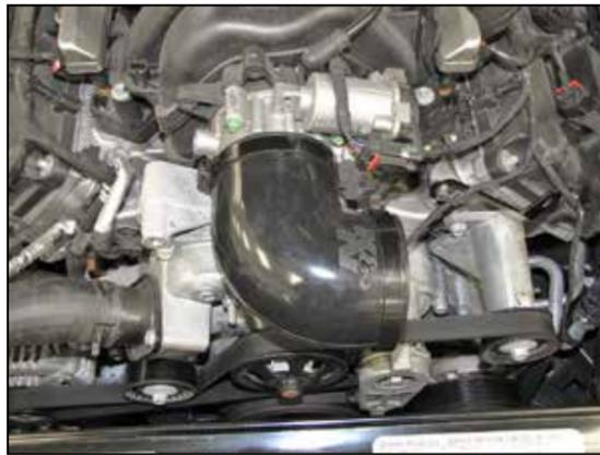
14. Install the provided 90° coupling hose (084088) onto the throttle body and secure with the provided hose clamps
